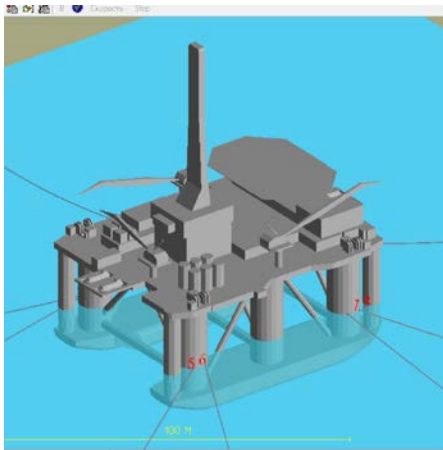
Fig. 2 Three-dimensional geometric model of a floating object in the program «Anchored Structures»
