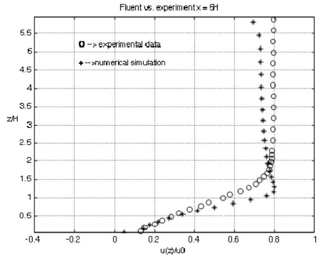
Figure 5b Mean velocity profile  $x = 5H$
