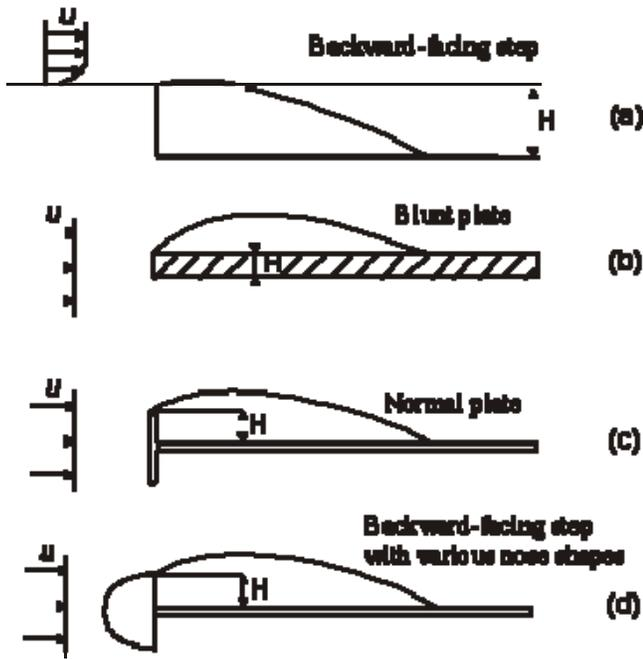
Figure 1 Flow configurations with separation and reattachment
