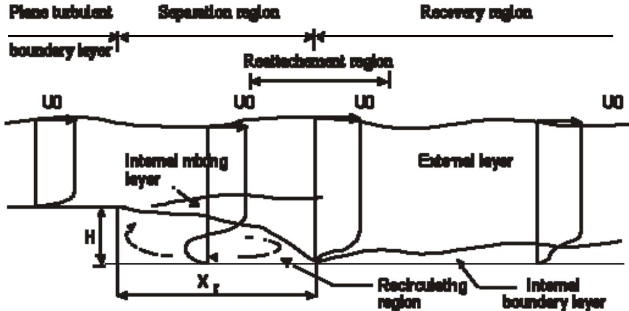
Figure 2 Flow configuration
