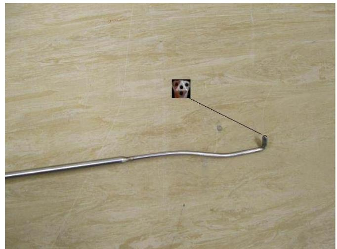
Fig. 3 Four-hole Cobra probe
