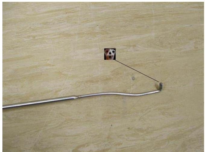
Fig. 3 Four-hole Cobra probe
