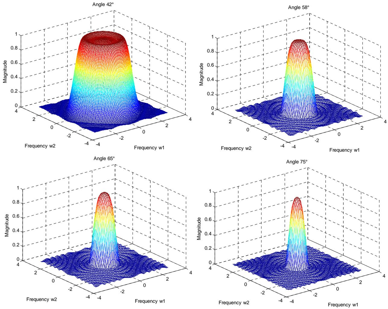
Fig. 5 The 3-D magnitude responses obtained for  $\omega_3=\omega_0$  and different angles  $\theta$  (42°, 58°, 65°, and 75°)
