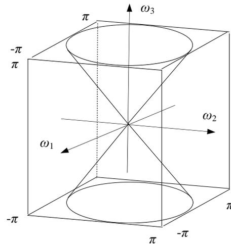
Fig. 1 The ideal frequency response of a cone filter (with  $\gamma=1$ )
