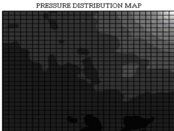
Fig.5. Result pressure distribution map. The injection well is at the NE end, the production well is at SW end. The pressure variation is due to the fracture distribution.
