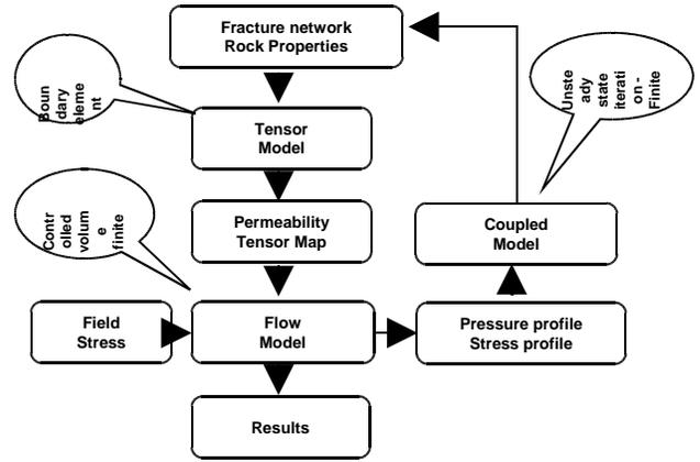
Fig. 1: Coupled simulation for stress-dependent DFN.
