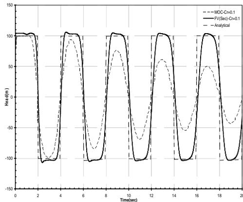
Fig 2. Variations in hydraulic head at the valve (Test I) for MOC, FVM and analytical solution
