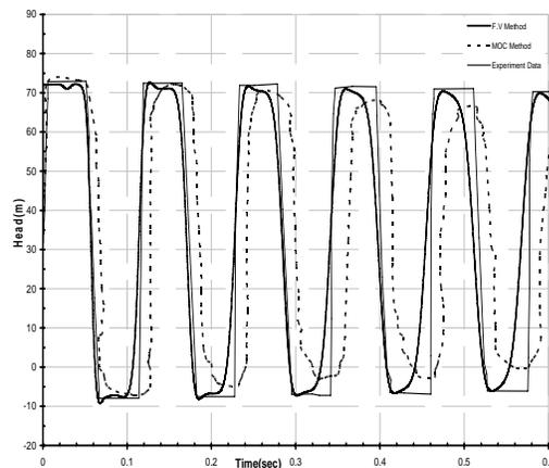
Fig 4. Variations in hydraulic head at the valve (Test II) for MOC and FVM and laboratory data ( $Cr=0.5$ )
