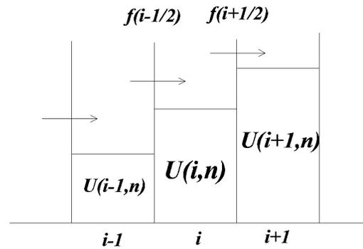
Fig 1. Finite Volume Stencil
