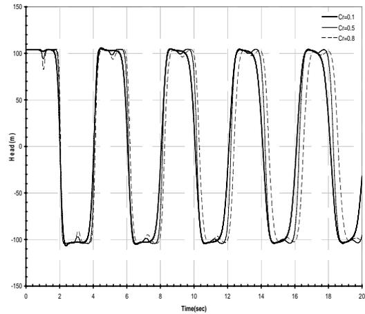
Fig 3. Pressure head traces at valve (Test I) for various Cr No.(FVM)
