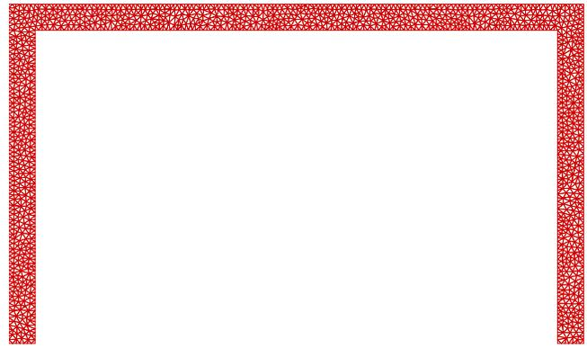
Fig.13. unstructured mesh applied for GFVM solver
