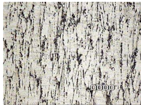
Fig. 8 Microstructure of extruded specimen after etching(100X)
