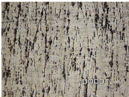
Fig. 6 Microstructure of extruded specimen before etching(100X)
