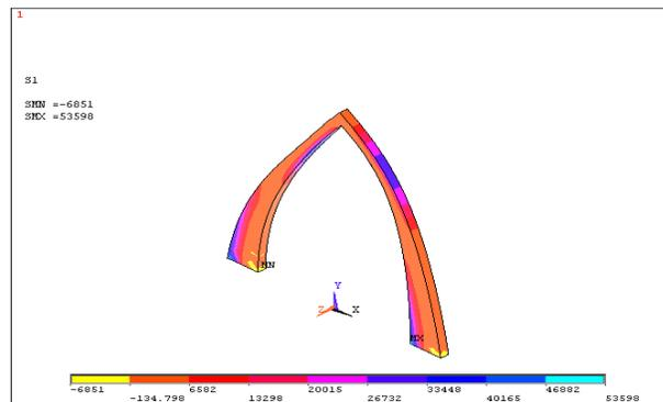
Fig III: Catenary arch modeling by ansys
