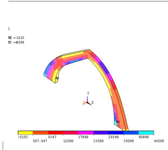
Fig VII: Catenary arch modeling by ansys
