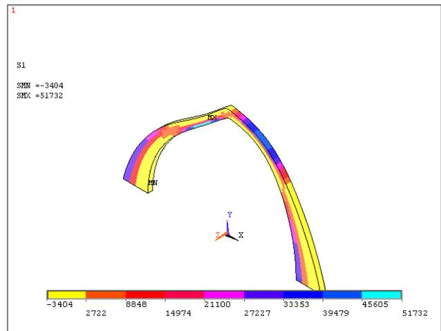
Fig V: Obtuse angle arch modeling by ansys
