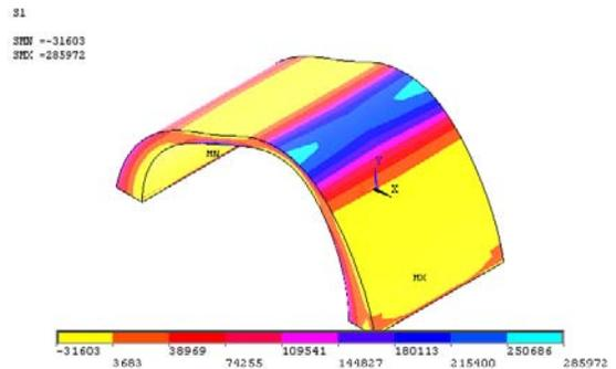
FigXII:semicircular arch with 4m spam and the place of stresses( $N / m^2$ )
