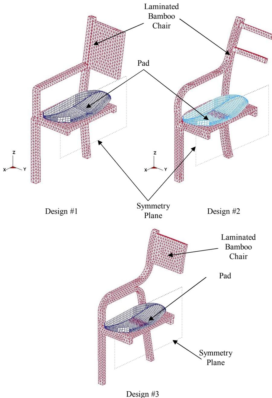
Fig.3. Isometric view of FEA models in static analysis
