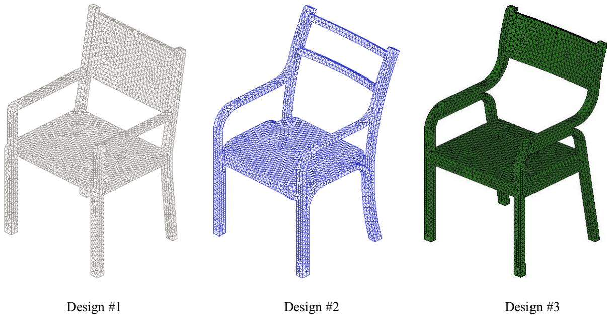
Fig.1. Design models of laminated bamboo chair
