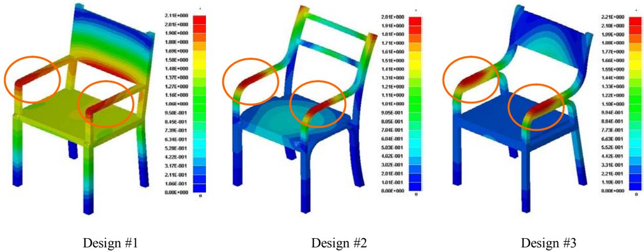
Fig. 18. Distribution of total displacement (in mm) in impact analysis
