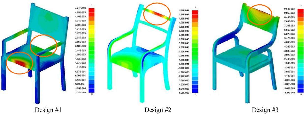
Fig.16. Distribution of displacement in Z-direction (in mm) in dynamic analysis
