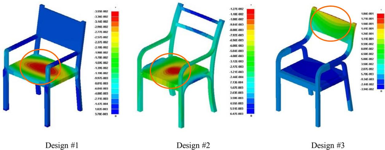
Fig.13. Distribution of displacement in Z-direction (in mm) in static analysis
