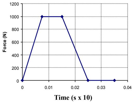
Fig.6. Applied pad force for static loading
