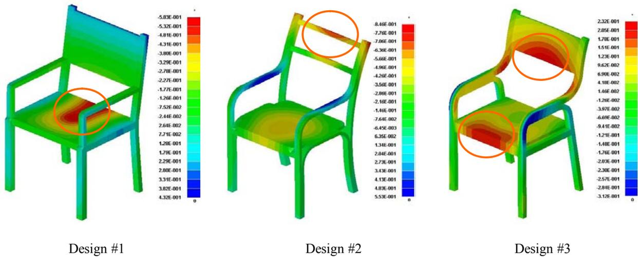
Fig. 19. Distribution of displacement in Z-direction (in mm) in impact analysis
