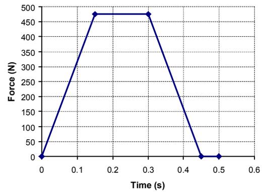
Fig.7. Applied pad force for dynamic loading
