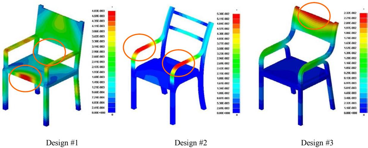
Fig.15. Distribution of total displacement (in mm) in dynamic analysis
