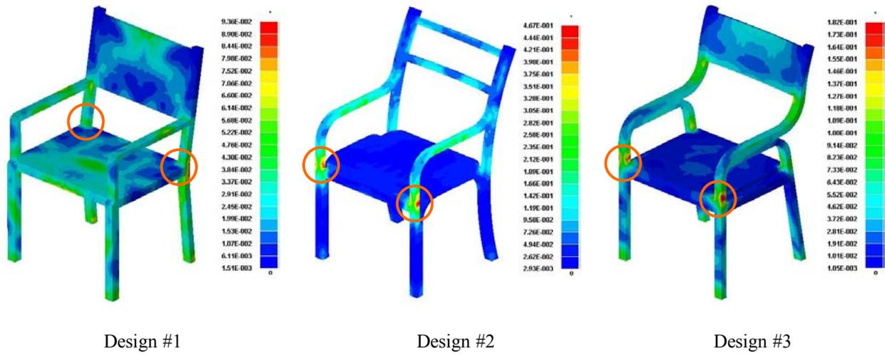
Fig.14. Distribution of maximum *von Mises* stress (in MPa) in dynamic analysis
