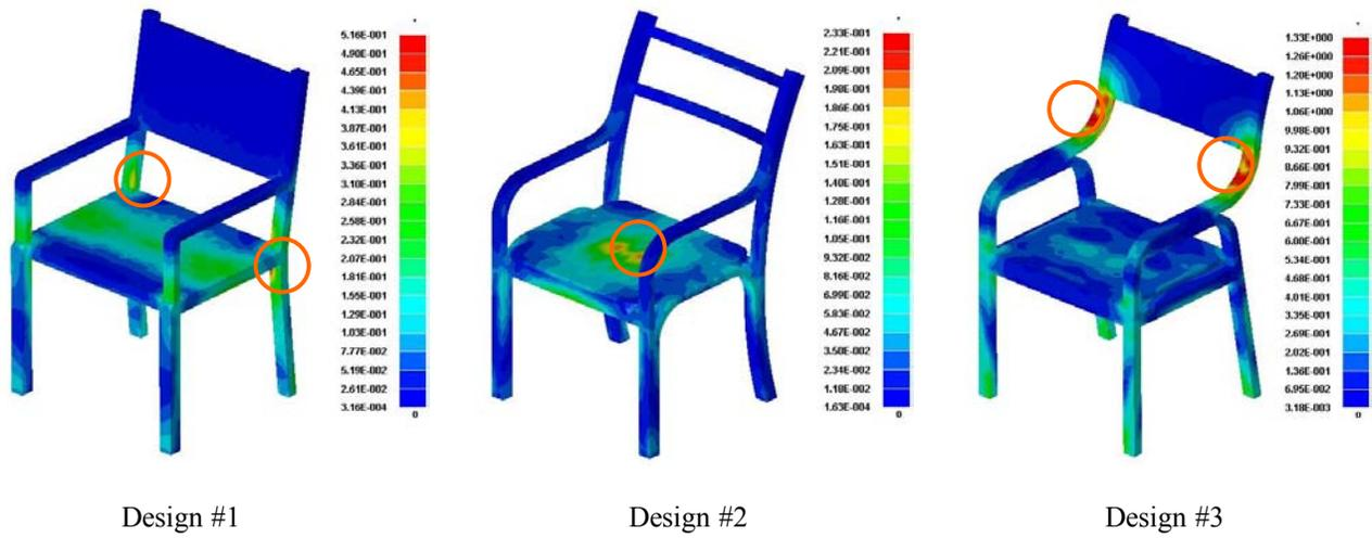
Fig.11. Distribution of maximum *von Mises* stress (in MPa) in static analysis
