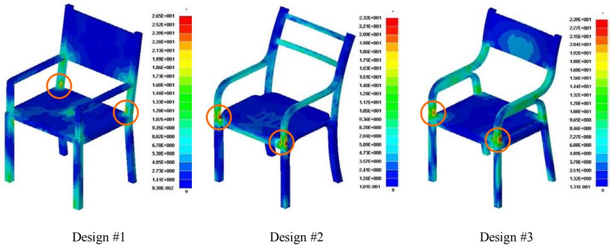
Fig. 17. Distribution of maximum *von Mises* stress (in MPa) in impact analysis
