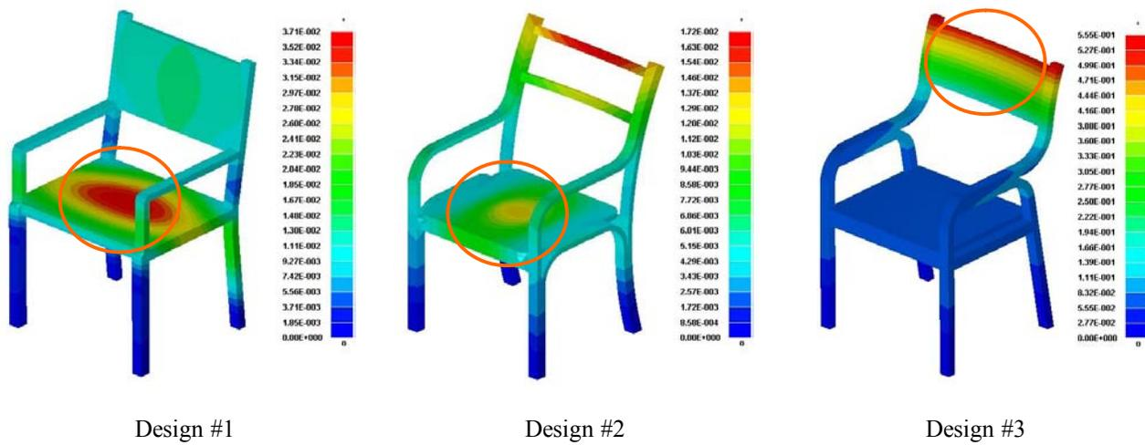
Fig.12. Distribution of total displacement (in mm) in static analysis
