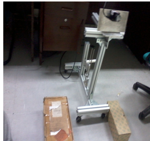
Fig. 10: show the platform and laser range finder setup
