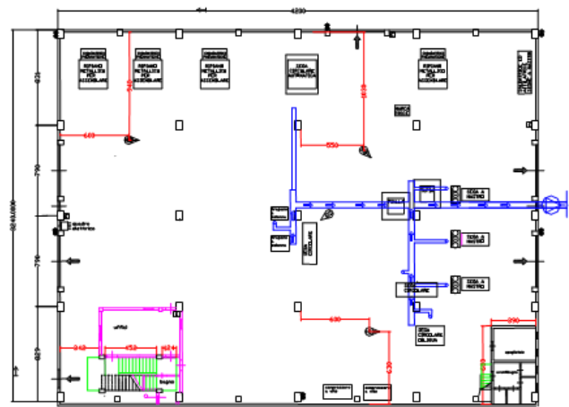
Fig. 1: Layout of the working area. The blue line represents the powder aspirator, while the various boxes are the different machineries. The purple area is the administrative office.
