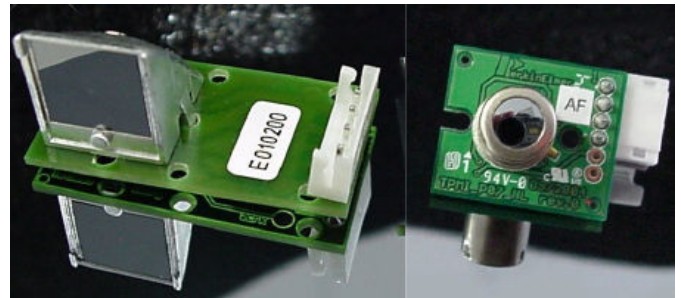
Fig. 7. Photographs of manufactured types of sensors of medium radiation temperature
