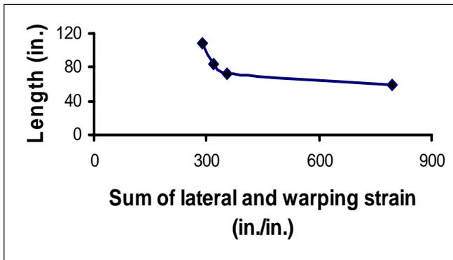
Figure 5. Length versus sum of lateral and warping strains
