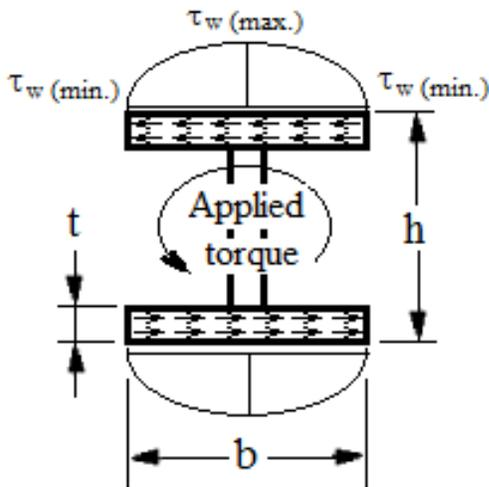
Figure 6. Cross-sectional of a beam with illustrated maximum warping stress.
