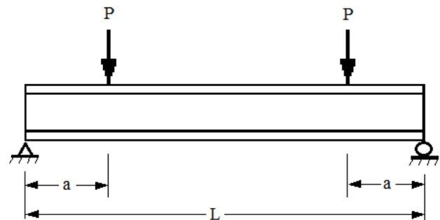
Figure 1. Beam and loading
