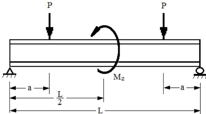
Figure 2. Combined Bending and Applied Torsion
