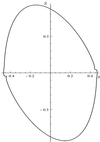
Fig. 10. Cart velocity vs. cart displacement for piecewise linear friction model - case 2.
