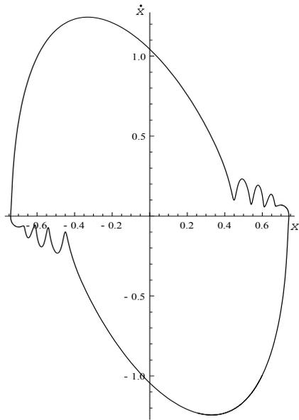
Fig. 4. Cart velocity vs. cart displacement for continuum non-linear friction model.
