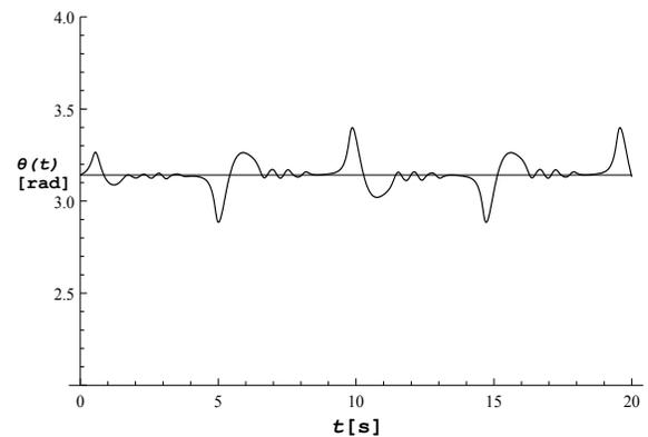
Fig. 3. Pendulum displacement vs. time for continuum non-linear friction model.
