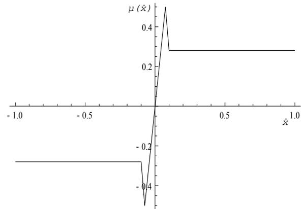
Fig. 8. Piecewise friction linear characteristic - case 2.
