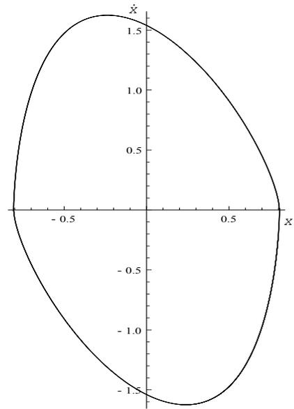
Fig. 13. Cart velocity vs. cart displacement for piecewise linear friction model - case 3.
