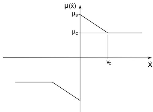
Fig. 14. Piecewise friction characteristic model.
