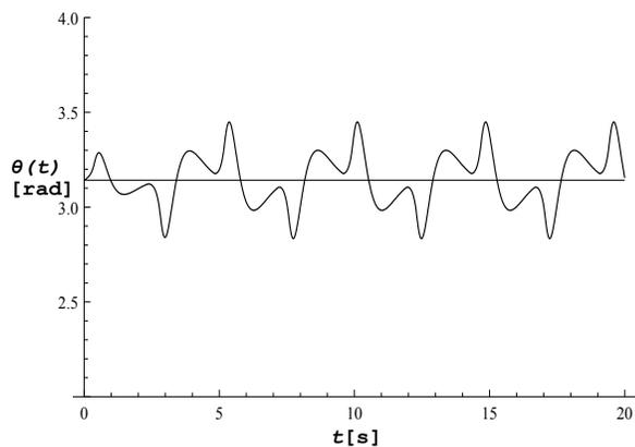
Fig. 12. Pendulum displacement vs. time for piecewise linear friction model - case 3.
