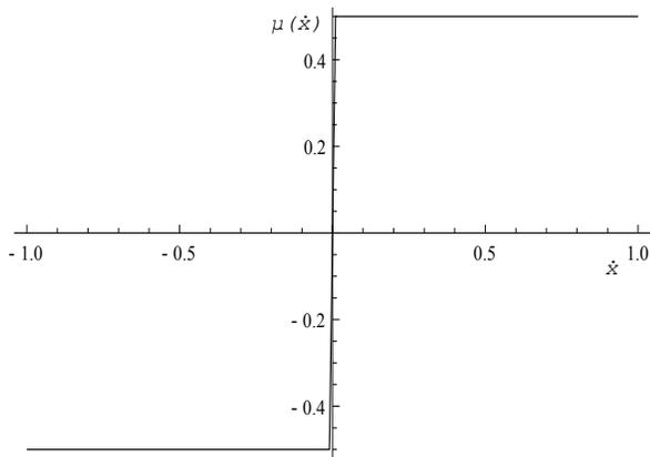
Fig. 11. Piecewise friction linear characteristic - case 3.
