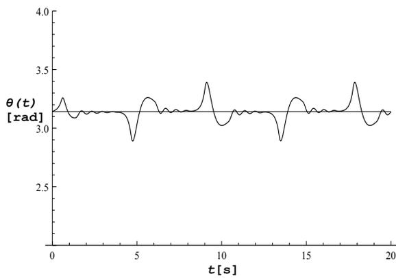
Fig. 6. Pendulum displacement vs. time for piecewise linear friction model - case 1.
