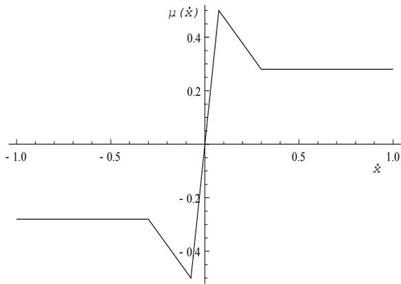
Fig. 5. Piecewise friction linear characteristic - case 1.
