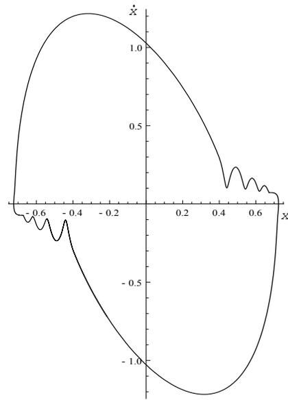
Fig. 7. Cart velocity vs. cart displacement for piecewise linear friction model - case 1.
