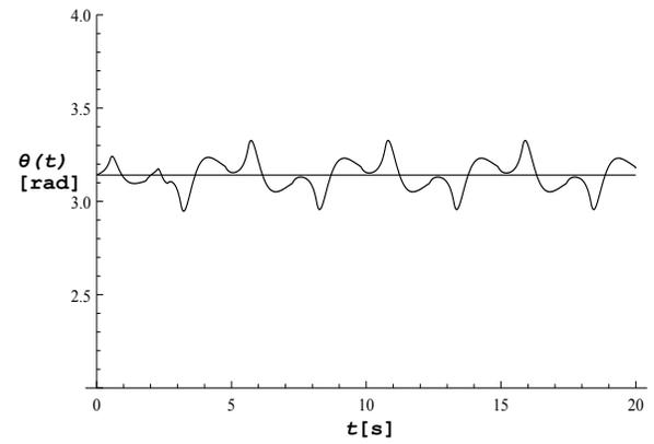
Fig. 9. Pendulum displacement vs. time for piecewise linear friction model - case 2.
