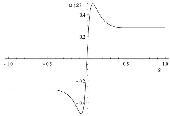
Fig. 2. Non-linear friction characteristic.
