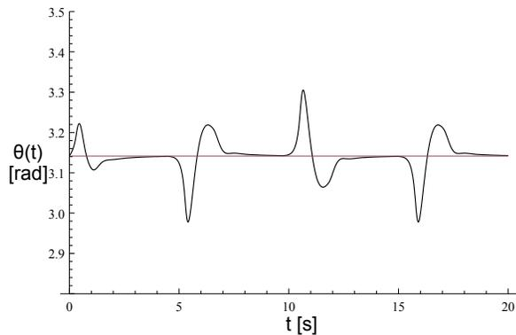
Fig. 15. Pendulum displacement vs. time for  $\mu_S = 0.3$  and  $\mu_C = 0.2$ .
