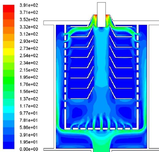
Fig.14 Velocity magnitude field of Nitrogen (10%)
