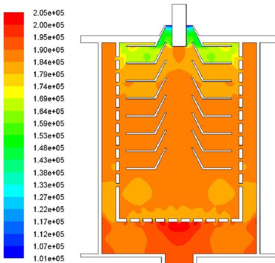
Fig.16 Static pressure field of mixture (10%)
