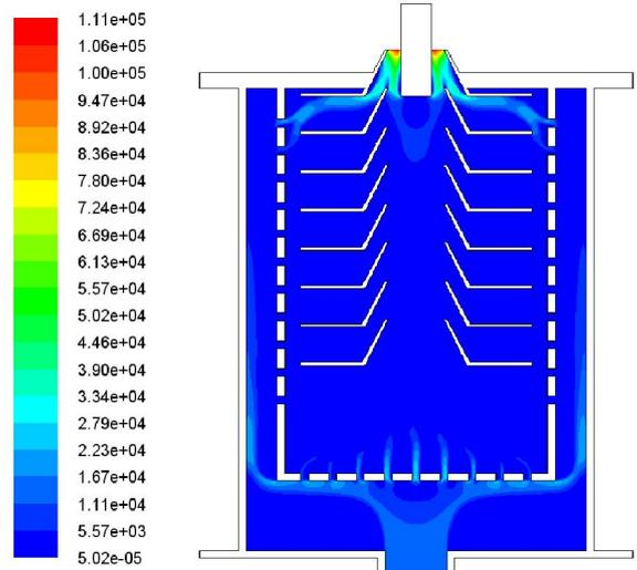
Fig.7 Dynamic pressure field of mixture (10%)
