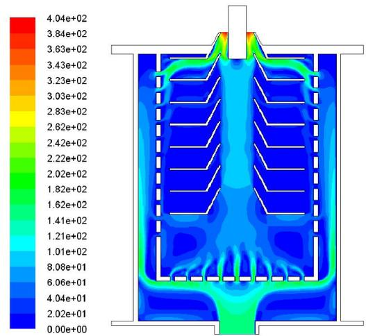
Fig.18 Velocity magnitude field of mixture (1%)
