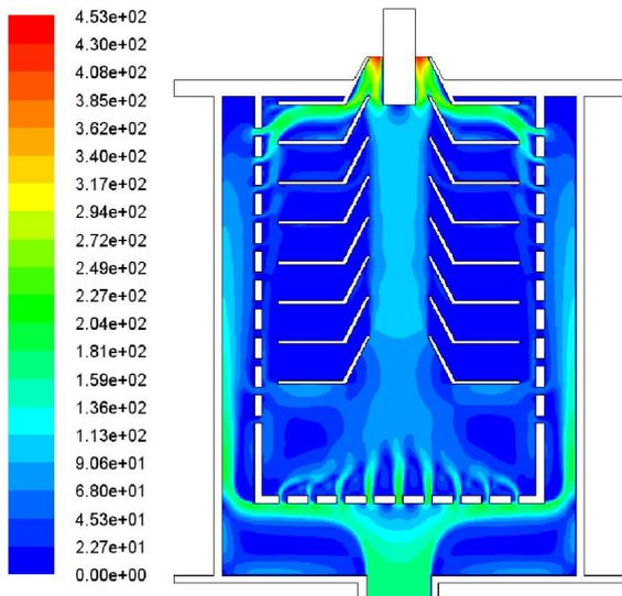
Fig.3 Velocity magnitude field of mixture (10%)
