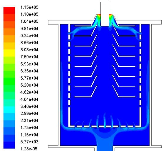
Fig.12 Dynamic pressure field of mixture (1%)
