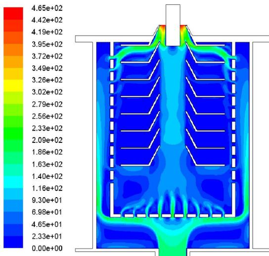
Fig.5 Velocity magnitude field of spray water (10%)
