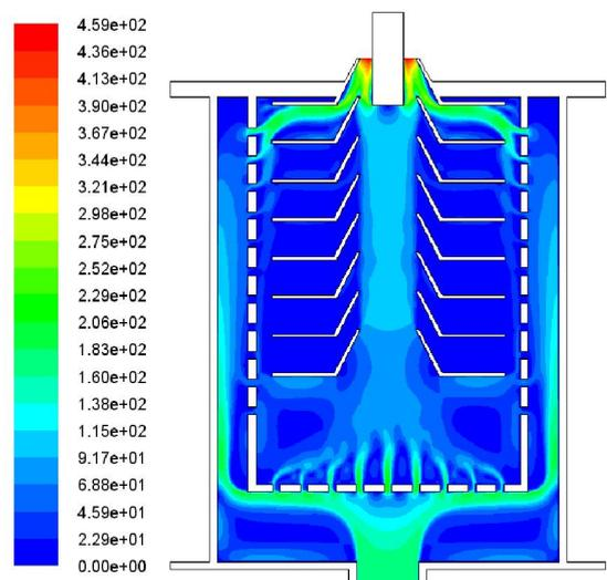
Fig.8 Velocity magnitude field of mixture (1%)
