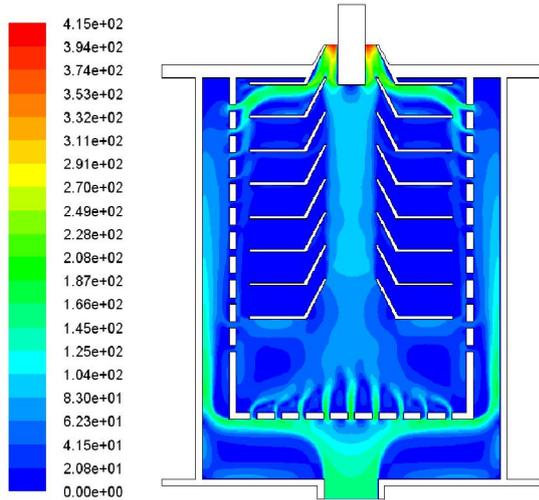
Fig.20 Velocity magnitude field of spray water (1%)
