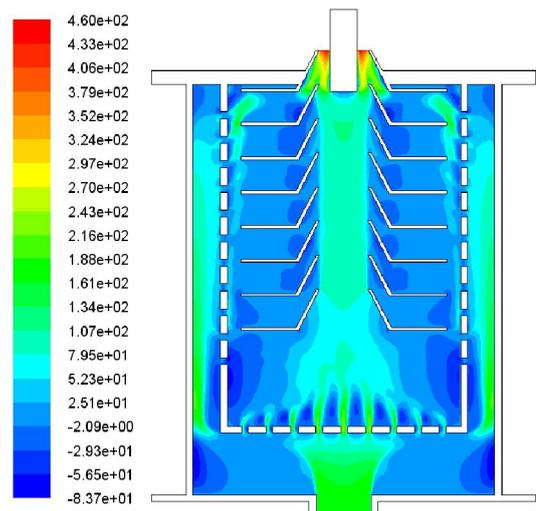
Fig.23 Z direction velocity field of mixture (1%)
