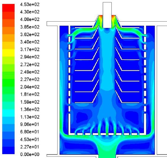
Fig.4 Velocity magnitude field of Nitrogen (10%)
