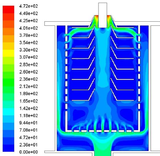
Fig.10 Velocity magnitude field of spray water (1%)
