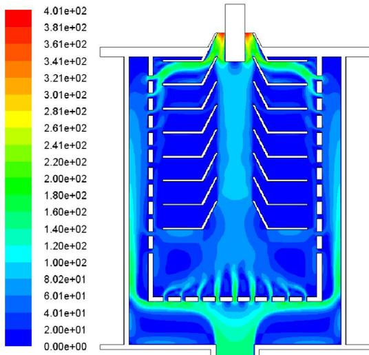
Fig.15 Velocity magnitude field of spray water (10%)
