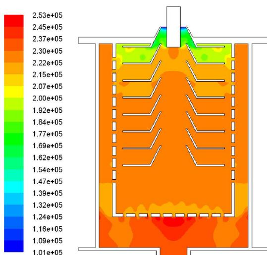
Fig.11 Static pressure field of mixture (1%)
