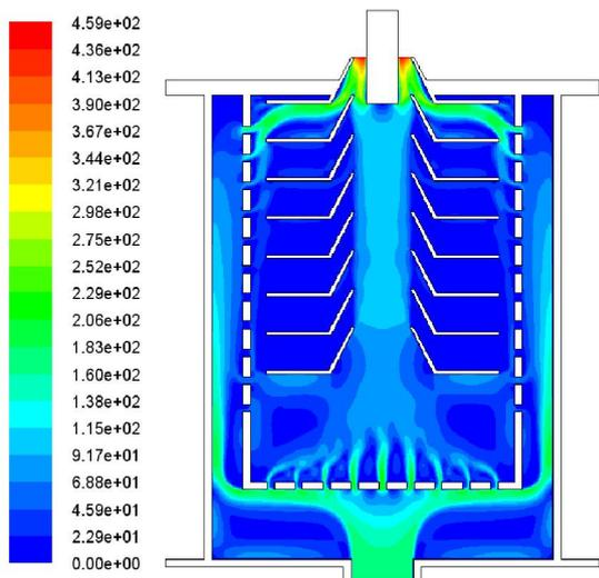
Fig.9 Velocity magnitude field of Nitrogen (1%)
