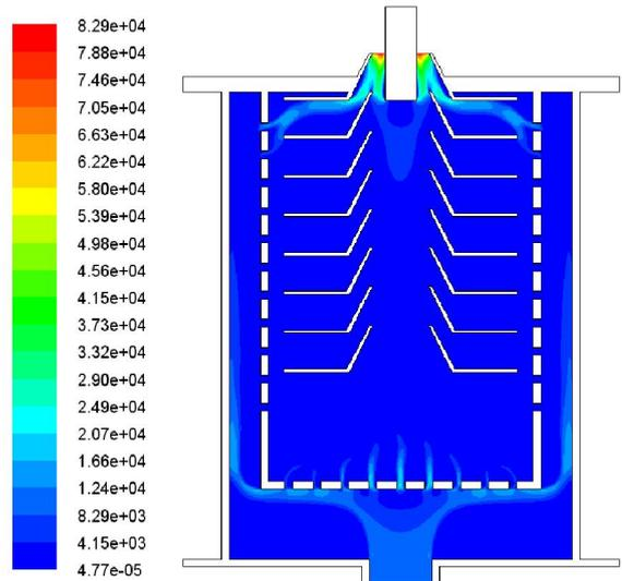
Fig.17 Dynamic pressure field of mixture (10%)
