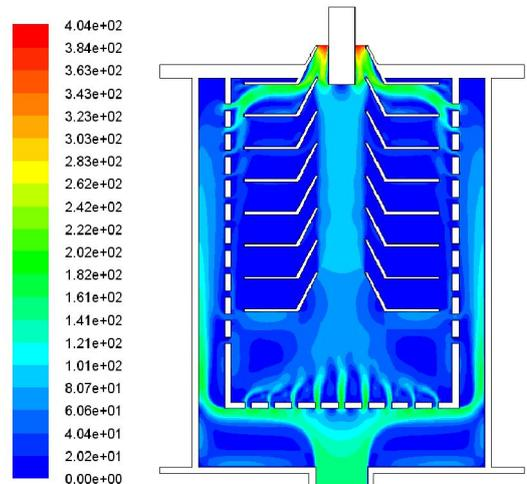
Fig.19 Velocity magnitude field of Nitrogen (1%)
