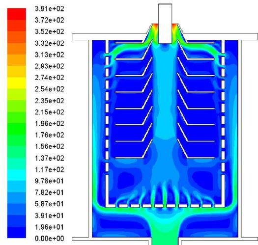
Fig.13 Velocity magnitude field of mixture (10%)
