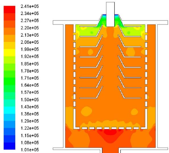
Fig.6 Static pressure field of mixture (10%)
