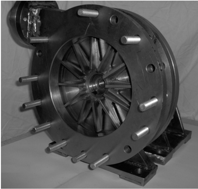
Fig. 2. View of the pump flow system. The front wall of the casing and impeller nut were dismantled
