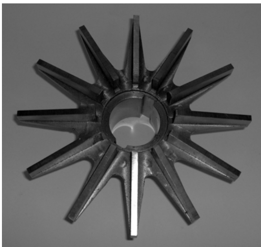
Fig 3. The impeller of the pump – view
