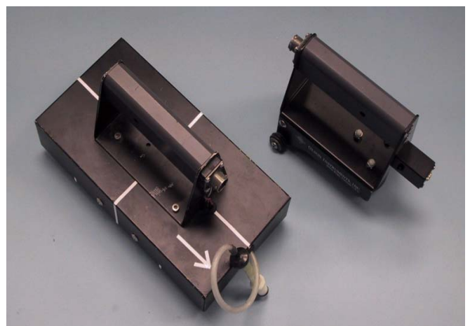
Fig. 2 Top view of IE equipments of Olson Engineering, Inc., in which the left is the IE scanner used for NDE360 and the right the traditional IE unit used for CTG (Courtesy of L.D. Olson).
