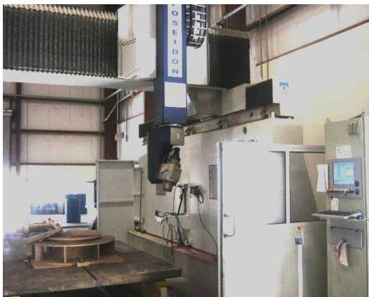
Figure.7 CMS –Poseidon specific purpose 5-axis CNC Machine used for machining sand moulds
