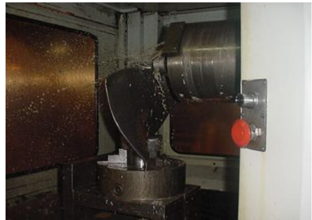
Figure.9. Top radius profile machining on 4-axis HMC
