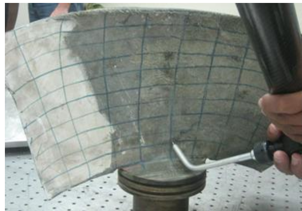
Figure.3 Digitizing the blade surface with point probe
