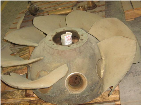
Figure.2 Worn out blades in the hub assembly
