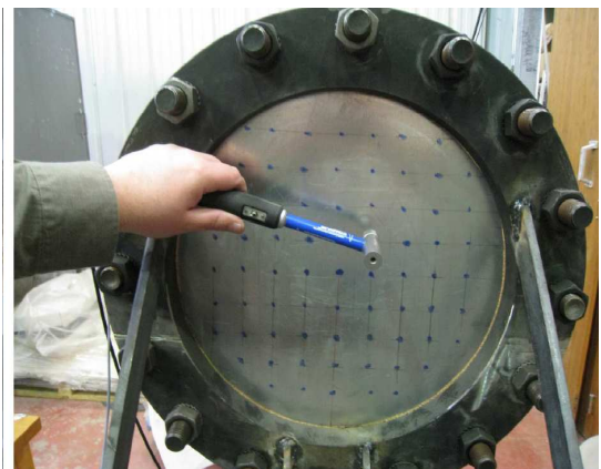
Fig.13 Experimental set-up for impact location
