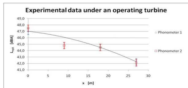
**Fig. 15:** Experimental data taken in proximity of an operating wind turbine. The receiver is placed at 1,5 m and the phonometers have been placed along two radius pointing to the turbine base.
