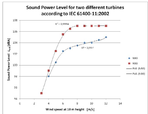
**Fig. 4:** Sound Power Level data fit for two different turbines. Data have been provided by manufacturer datasheets. The  $R^2$  determination coefficient of the fit is reported in the plot.
