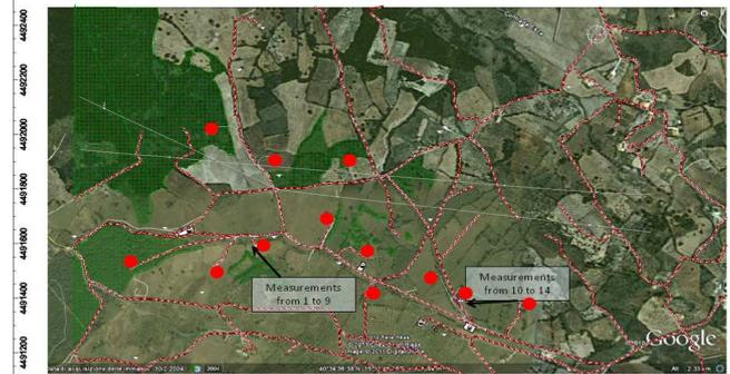
**Fig. 14:** Map of the area of Taverne Vecchie (SA), Italy, taken from Google map. The map has been implemented in CadnaA framework and the roads have been traced. The turbines are the red circles.
