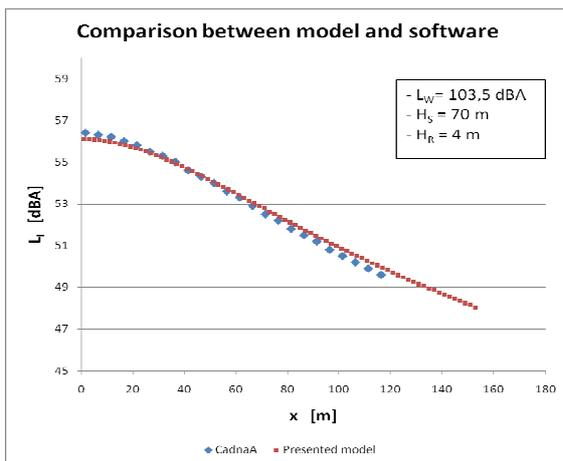
**Fig. 13:** comparison between noise level predicted with CadnaA (blue diamonds) and with the proposed model (red squares), for a pointlike source with  $L_W= 103,5$  dBA, height = 70 m and absorbing ground. The values are taken at 4 m of height.
