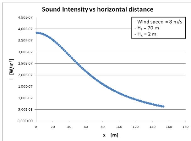
**Fig. 5:** Sound Intensity vs horizontal distance from the turbine base for a pointlike source with  $L_W= 103,5$  dBA, height of the source = 70 m and height of the receiver = 2 m.
