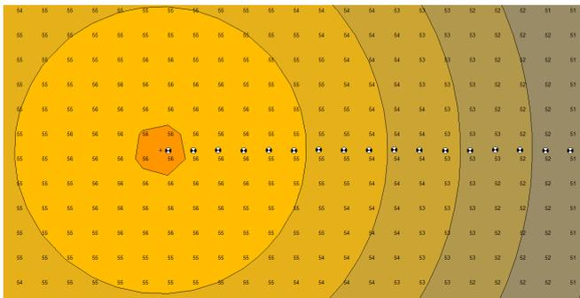
**Fig. 8:** CadnaA noise map (values are in dBA) for a pointlike source with  $L_W= 103,5$  dBA (wind speed = 8 m/s), height = 70 m, absorbing ground. The grid is evaluated at 2 m from the ground and the distance between two receivers (black and white circles) is 5 m, while their height is 4 m.
