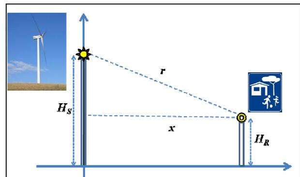
Fig. 2: Geometry of the source and receiver configuration.
