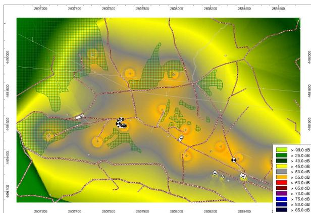
**Fig. 17:** Noise map simulation in an average wind speed condition, i.e. 8 m/s. The resulting source power is 103,5 dBA.
