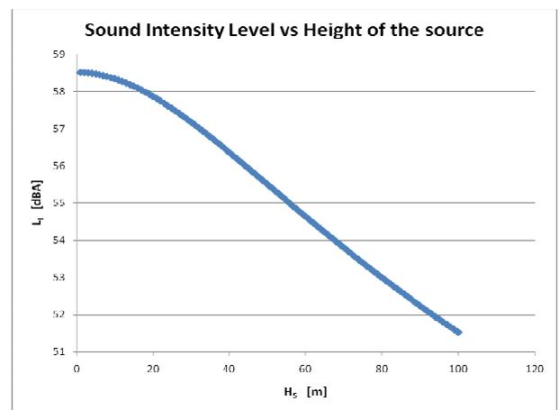
**Fig. 7:** Sound Intensity Level vs height of the source for a pointlike source with  $L_W= 103,5$  dBA, distance from wind turbine base = 70 m and height of the receiver = 2 m.
