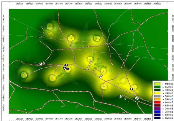
**Fig. 16:** Noise map of the wind farm area, obtained in predictive software framework. The power of the pointlike sources (turbines) has been set to 93,5 dBA, according to the experimental measurement taken.
