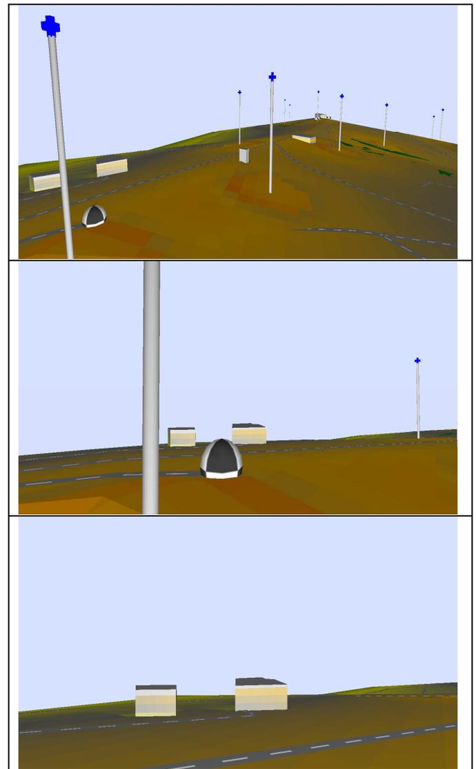
**Fig. 18:** 3D images of the wind farm area under investigation. The colours on the terrain are according to the noise pattern and the legenda in Fig. 17. The blu crosses are the pointlike sources, mimicking the wind turbines, the white and black circles are the receivers and the parallelepipeds are the buildings. The different colours on the buildings represent the noise level according to the legenda in Fig. 17.
