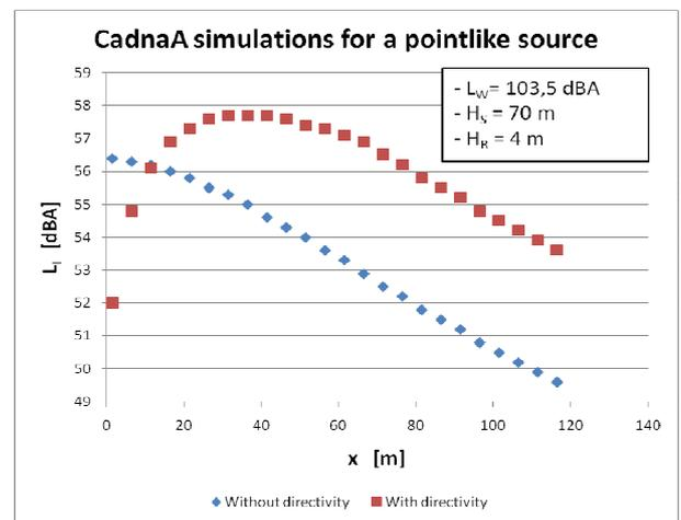
**Fig. 10:** CadnaA results for a pointlike source with  $L_W= 103,5$  dBA, height = 70 m and absorbing ground. The values are taken at 4 m of height and the plots are with or without directivity.
