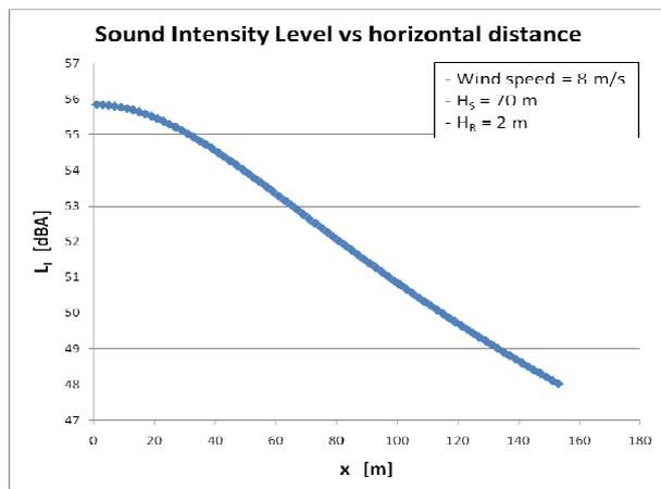
**Fig. 6:** Sound Intensity Level vs horizontal distance from the turbine base for a pointlike source with  $L_W= 103,5$  dBA, height of the source = 70 m and height of the receiver = 2 m.
