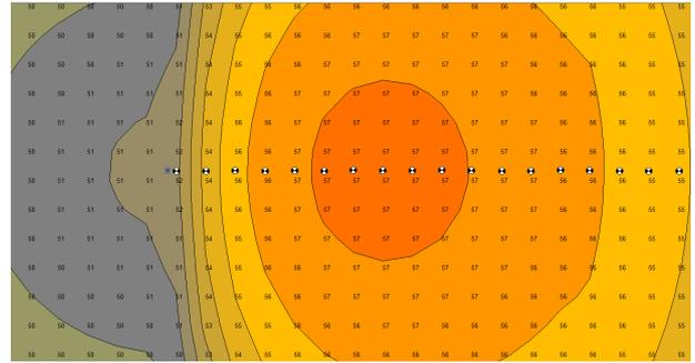
**Fig. 9:** CadnaA noise map (values are in dBA) for a pointlike source with  $L_W= 103,5$  dBA (wind speed = 8 m/s), height = 70 m, absorbing ground and high directivity. The grid is evaluated at 2 m from the ground and the distance between two receivers (black and white circles) is 5 m, while their height is 4 m.
