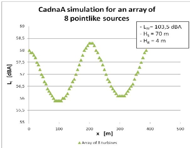
**Fig. 12:** CadnaA results for an array of 8 pointlike sources, limited to the proximity of three turbines, with  $L_W= 103,5$  dBA, height = 70 m and absorbing ground. Values are taken at 4 m of height and the data points refer to receivers shown in the previous map.
