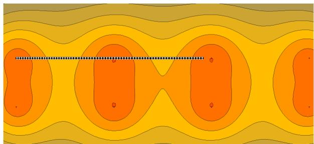
**Fig. 11:** CadnaA noise map for an array of 8 pointlike sources with  $L_W= 103,5$  dBA, height = 70 m and absorbing ground. The grid is evaluated at 2 m from the ground and the distance between two receivers (black and white circles) is 5 m, while their height is 4 m.
