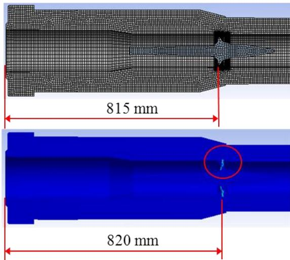
Fig.11 Projectile position before and after ramming – new barrel
