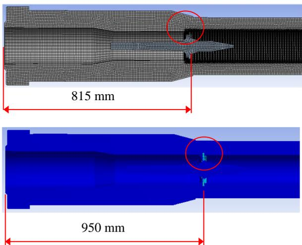
Fig.18 Projectile position – worn and heated barrel
