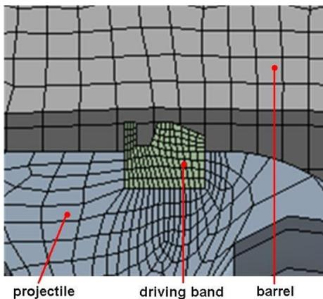
Fig.12 FEM model of driving band engraving
