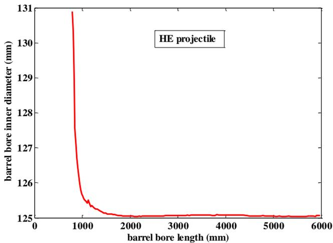
Fig.8 Wear of cannon barrel bore firing HE projectiles
