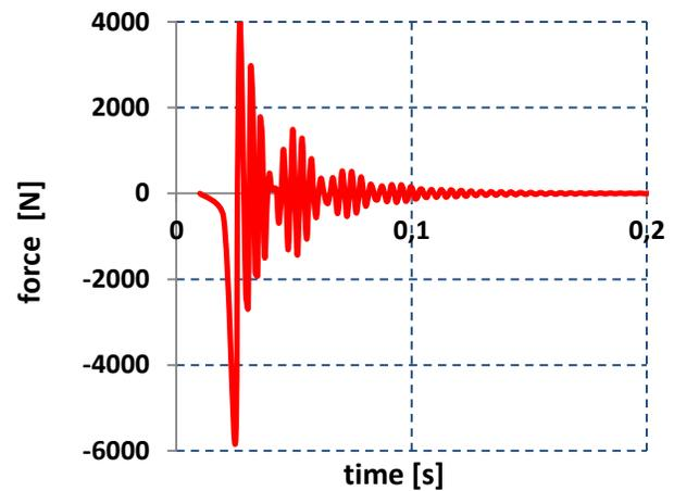
Fig.19 Reaction force in a worn barrel
