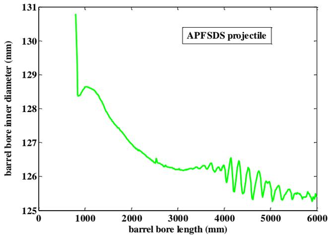
Fig.7 Wear of cannon barrel bore firing mainly APFSDS projectiles with ferrous sabot
