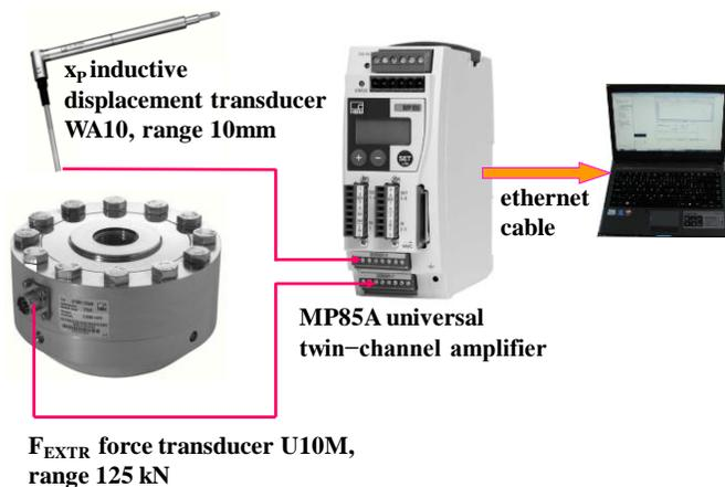
Fig.16 Scheme of measuring device
