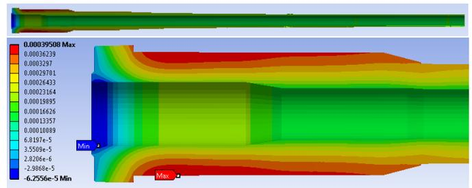
Fig.5 Radial thermal deformation field (m) of barrel wall
