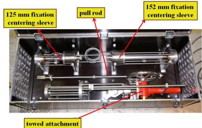
Fig.15 Force measurement device
