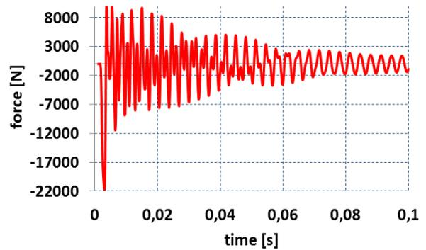
Fig.13 Reaction force in a new barrel
