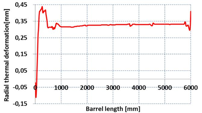
Fig.6 Barrel radial thermal deformation of the inner surface along the barrel length
