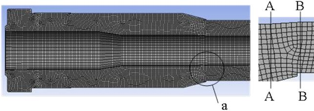
Fig.3 Model of a 125 mm tank cannon barrel
