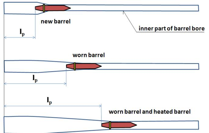
Fig.10 Explanation of projectile position in different barrels
