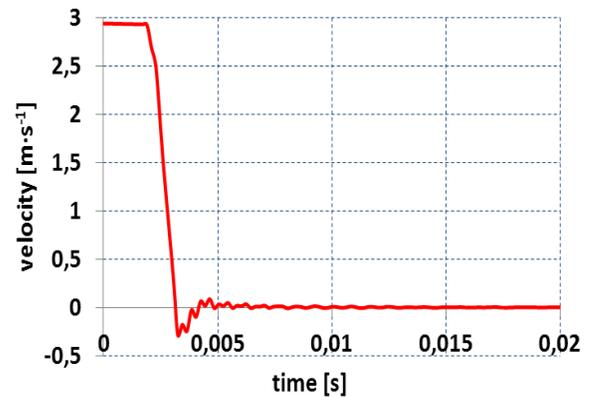
Fig.14 Projectile velocity in a new barrel
