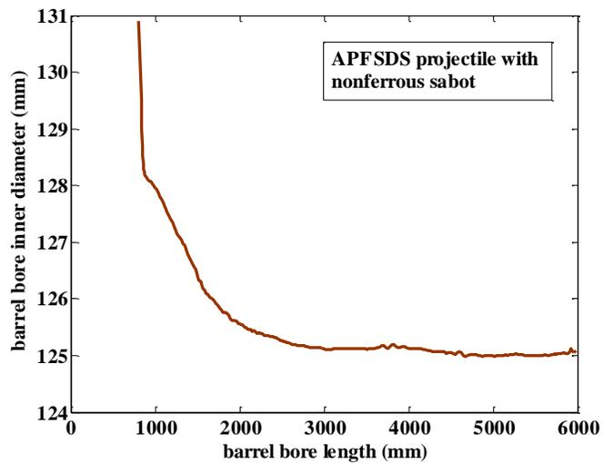
Fig.9 Wear of cannon barrel bore firing mainly APFSDS projectiles with nonferrous sabot
