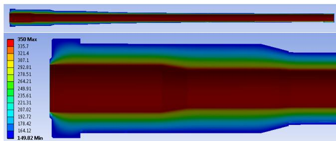
Fig.4 Temperature field in barrel wall
