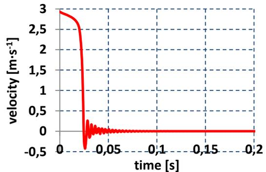
Fig.20 Projectile velocity in a worn barrel
