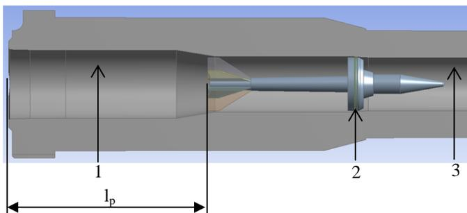
Fig.2 Position of the APFSDS projectile in the barrel after ramming: 1- chamber; 2- contact area between the forcing cone and the driving band; 3- leading part
