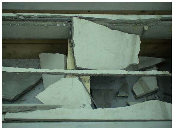
Fig. 9 Test specimen “C”: failure mechanism
