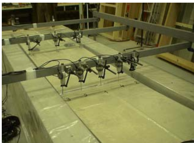
Fig. 3 Illustration of loading tests realized using vacuum loading test method
