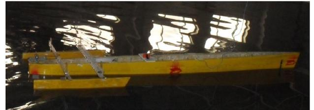
Fig.3 Free damping rolling test
