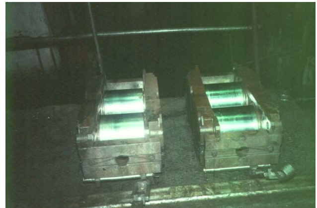
Fig.8 Carriages with support rolls of tube mill KHPT-250
