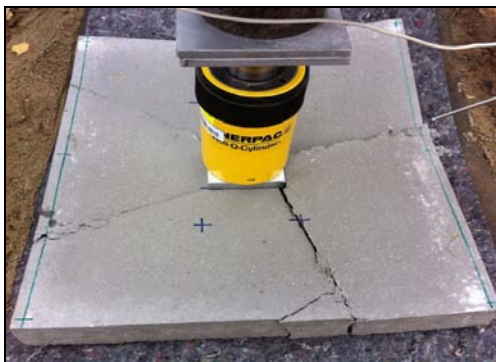
Fig. 4 Failure of the slab
