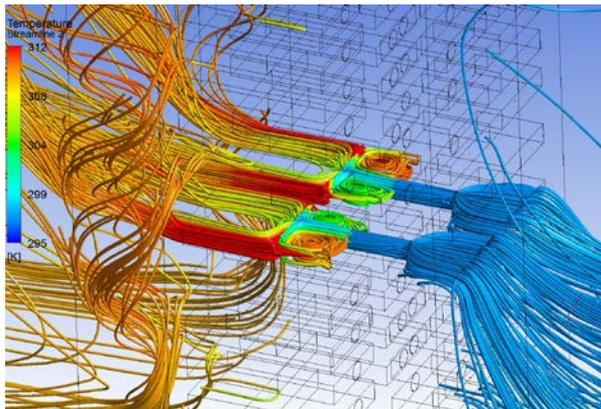
**Figure 13.** Detail of flow field in a simplified model of heat simulator with just two fans.
