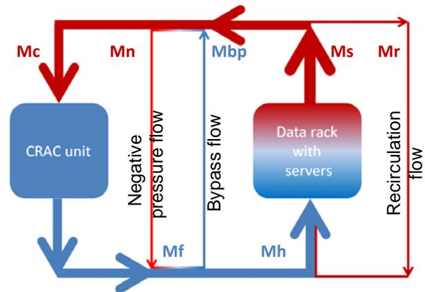
**Figure 1.** Data center air distribution. CRAC unit—computer room air conditioning unit.
