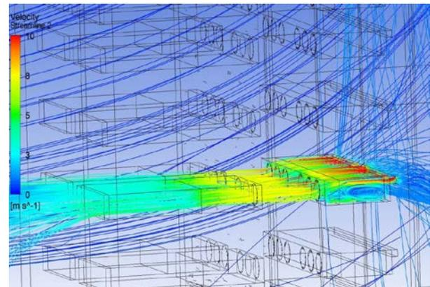
**Figure 14.** Detail of flow field in modified model of heat simulator with six fans.
