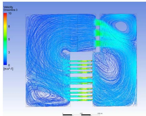
**Figure 20.** Missing 2U blending plate. Streamline in whole volume of model case with two chillers placed above data rack, color of streamline indicates air velocity.
