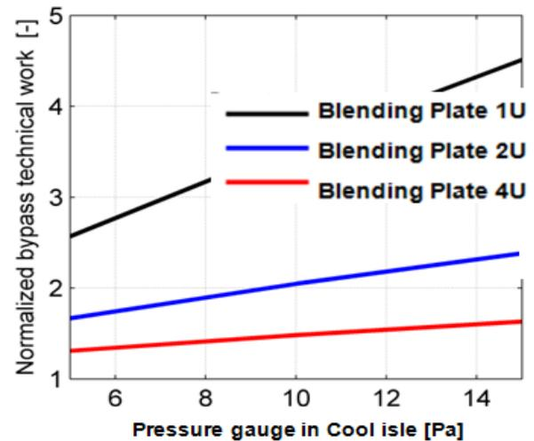
Figure 18 Dependence of increasing technical work on size of missing blending plate
