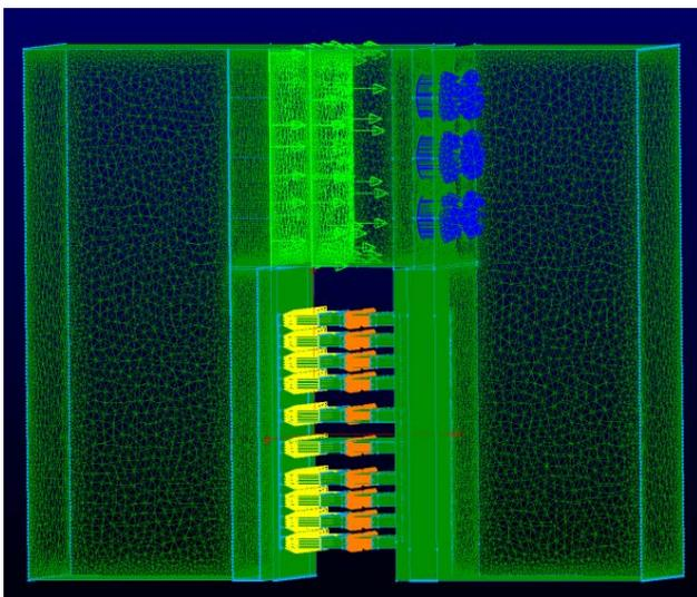
**Figure 9.** View of simulated volume. Numerical network with boundary conditions. "Chillers" are marked green, "fans" blue, "fans inside the heat simulators" orange, surfaces simulating heat of processors are marked yellow
