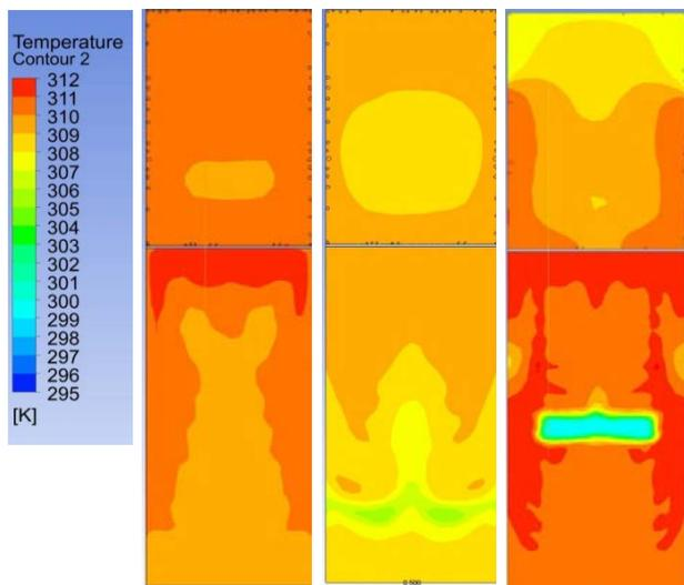
**Figure 21.** Temperature field at the outlet of servers (lower part) and temperature field at the inlet to the chiller (upper part) for each tested variants. From the left: completely separated cold and hot aisle, switched-off bottom server, missing blending plate inside the data rack.
