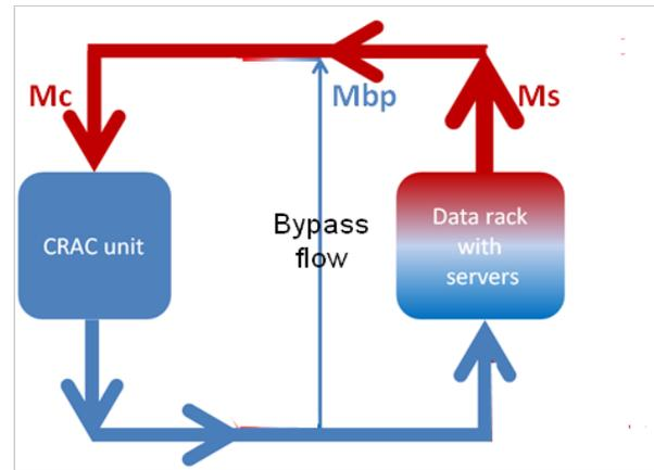
**Figure 16** Simplified flow in the data center
