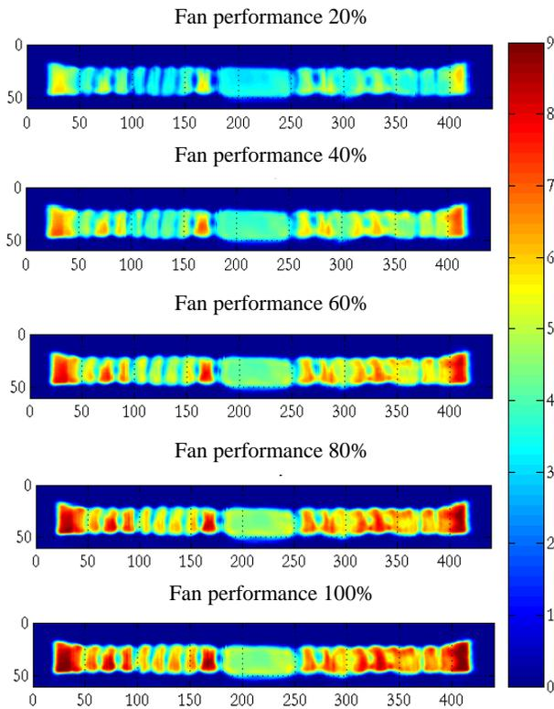
Figure 6. Outflow velocity from heat simulator
