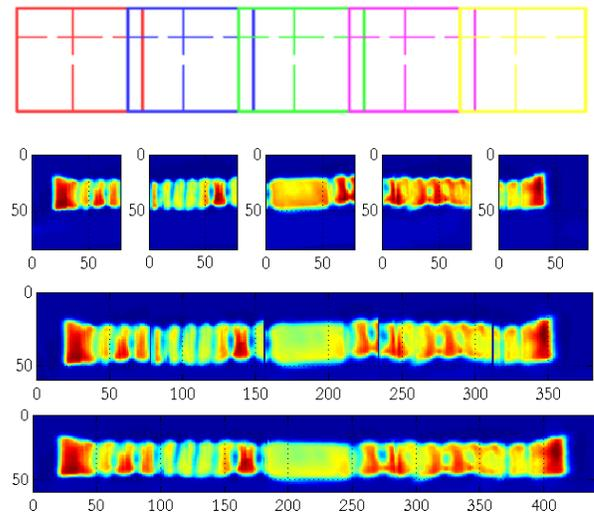
**Figure 5.** Division of velocity field at the outlet into five subregions, in which measurement using the stereo PIV method was subsequently carried out- first line. Raw result of five stereo PIV measurement-second line. Complete three dimensional velocity profile-third line. Final three dimensional profile.
