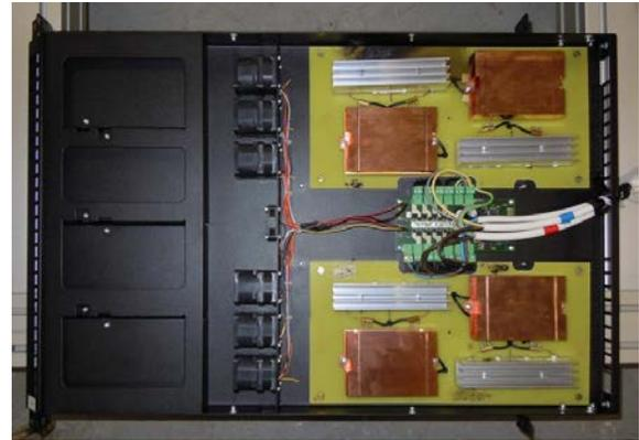
**Figure 4.** Heat simulator - model of server manufactured on the basis of ideological similarity with real server Supermicro 1026TT-IBQF.
