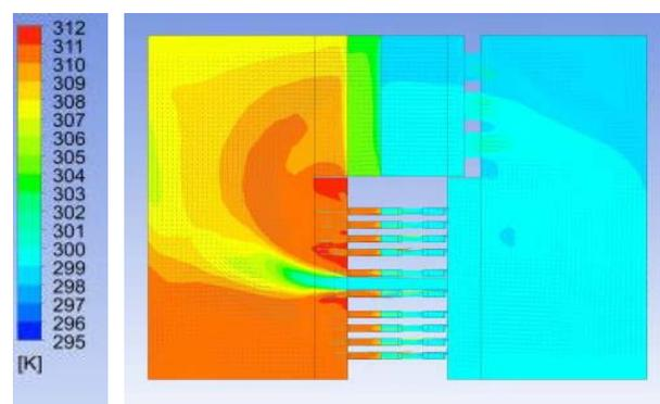
**Figure 22.** Field of temperature in cool and hot aisle. Effect of missing 2U blending plate
