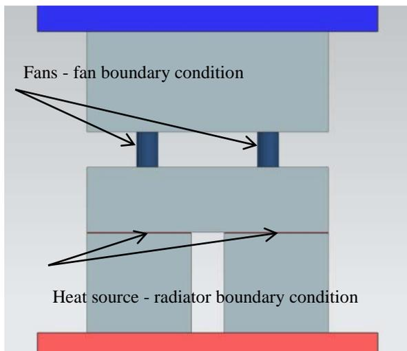
**Figure 11.** View of heat simulator. The simplified model with a pair of fans.
