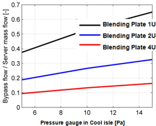
Figure 17 Dependence of increasing mass flow rate in bypass on size of missing blending plate
