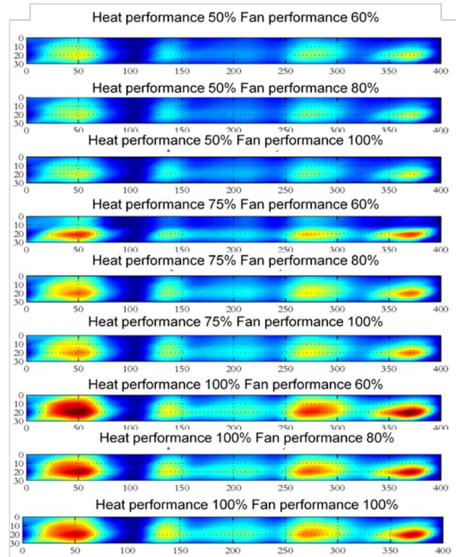
Figure 7 Temperature field at the outlet of heat simulator.
