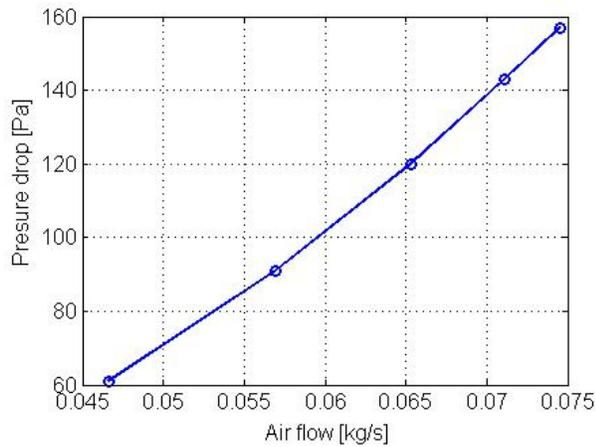
**Figure 8.** Relationship between flow Rate and pressure drop of heat simulator
