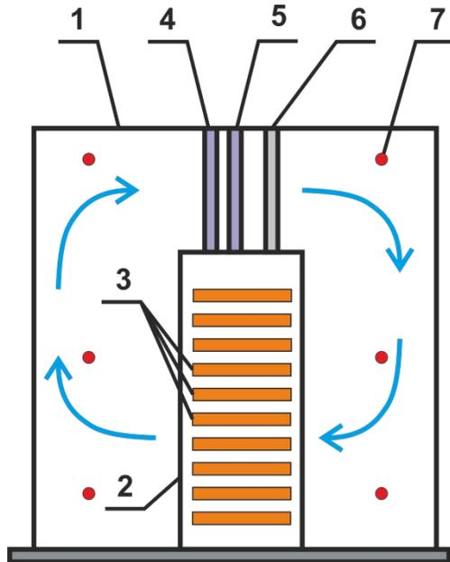
**Figure 3.** Real experiment simulating data center management, which was subsequently used as a model for numerical simulations. 1-Cold aisle (separated), 2- 27U data rack, 3-Server models, 4- High-temperature chiller, 5-Low-temperature chiller, 6-Group of six axial fans, 7-Hot aisle (separated)
