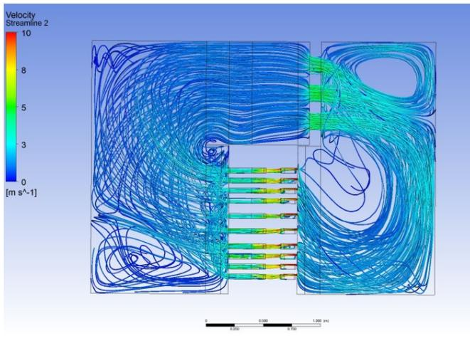
**Figure 19.** Completely close hot and cool aisle. Streamline in whole volume of model case with two chillers placed above data rack, color of streamline indicates air velocity.
