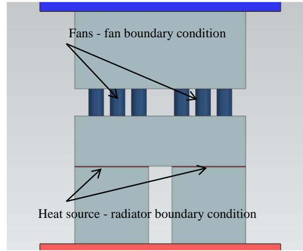
**Figure 12.** View of heat simulator. The modified model with six fans.
