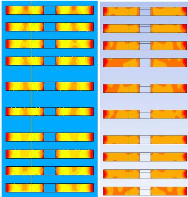
**Figure .15** Temperature field in plane of outlet of servers, first model of heat simulator in the left, new model in the right.
