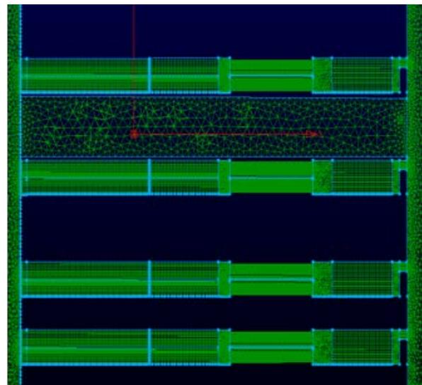
**Figure 10.** Detail of numerical mesh with missing blending plate.
