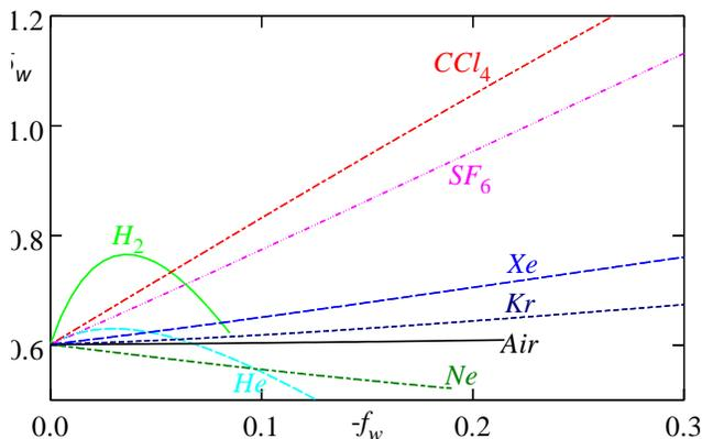
Fig.6: Mixture density at the wall  $\bar{\rho}_w$  versus injection factor  $-f_w$
