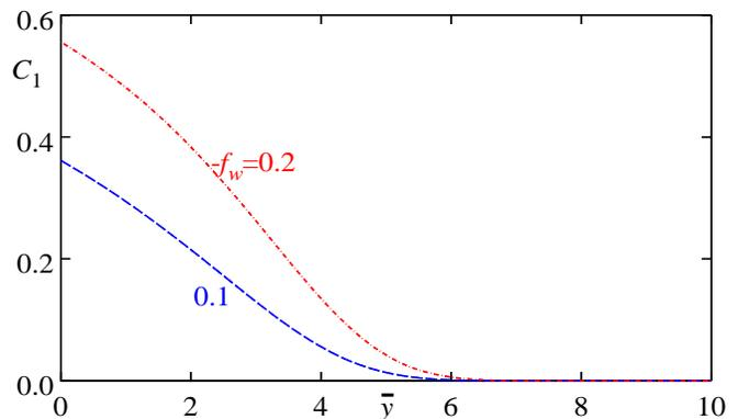
Fig.1: Distribution of the mass concentration of  $CCL_4$  across the boundary layer for two values of  $-f_w$ ;  $M = 2$ .
