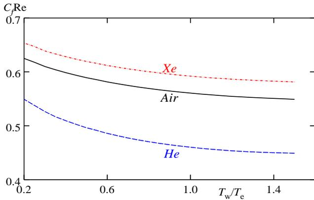
Fig.3: Normalized skin friction coefficient  $C_f Re$  versus wall temperature  $T_w/T_e$ ;  $M = 2$ ,  $-f_w = 0.1$ .
