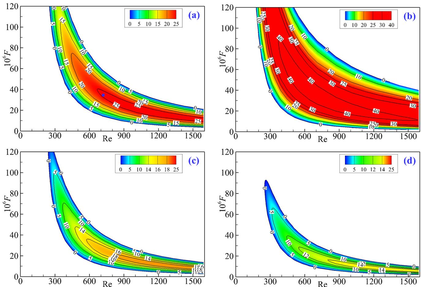
Fig.8: Mach=2 flat-plate boundary-layer stability-diagrams: nondimensional spatial amplification rate contours  $-\alpha_i = -\alpha_i(\text{Re}, F) \cdot 10^4$  for most unstable 3D perturbations with  $\chi = 60^\circ$ ; zero injection (a); injection of Air with  $-f_w = 0.1$  (b); injection of  $\text{CCl}_4$  with  $-f_w = 0.1$  (c) and injection of  $\text{CCl}_4$  with  $-f_w = 0.2$  (d).
