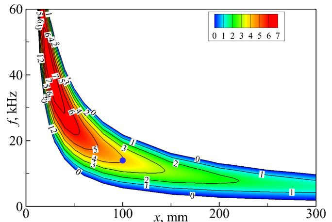
Fig.4: Mach=2 flat-plate boundary-layer zero-injection stability-diagram: dimensional spatial amplification rate contours  $-\alpha_i = -\alpha_i(x, f)$  [ $m^{-1}$ ] for 2D ( $\chi = 0^\circ$ ) perturbations.
