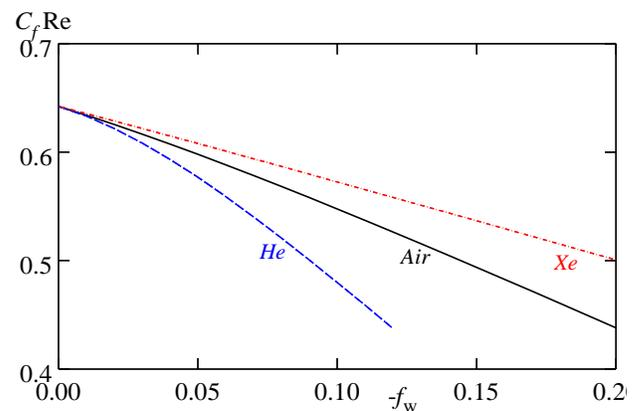
Fig.2: Normalized skin friction coefficient  $C_f \text{Re}$  versus injection factor for the adiabatic wall;  $M = 2$ .
