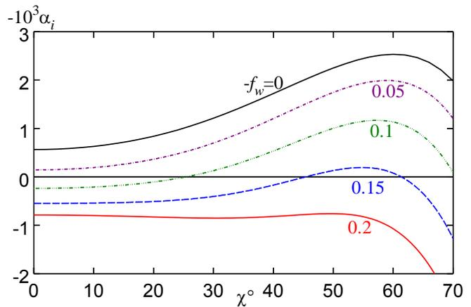
Fig.7: Nondimensional spatial amplification rates  $-\alpha_i$  for 3D perturbations versus angle  $\chi$ ; injection of  $CCl_4$ ,  $x = 100$  mm ( $Re = 720$ ),  $f = 14$  kHz ( $F \cdot 10^6 = 35$ )
