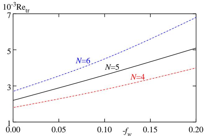
Fig.9: Transition Reynolds number  $Re_{tr}^N$  versus injection factor  $-f_w$  for  $CCl_4$ , as calculated by the  $e^N$ -method;  $M = 2$ .
