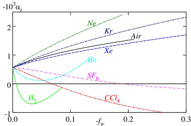
Fig.5: Nondimensional spatial amplification rate  $-\alpha_i$  of 2D perturbations versus injection factor  $-f_w$  for variety of foreign gases;  $Re = 720$ ,  $F \cdot 10^6 = 35$ .
