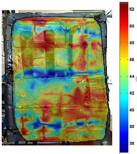
Fig. 34 Acoustic intensity, Final Foam
