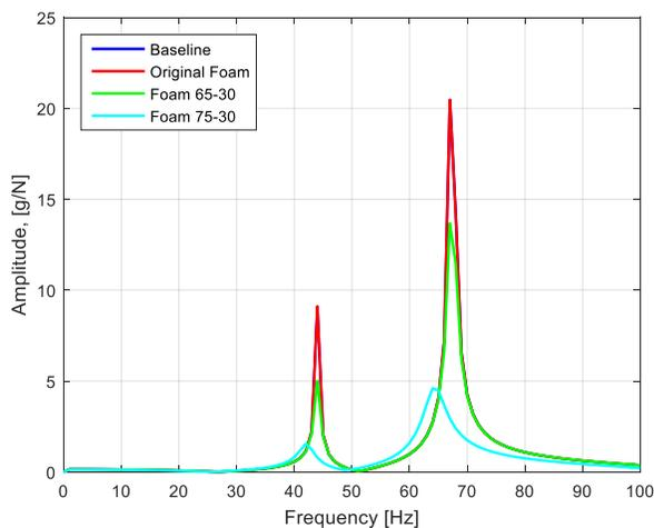
Fig. 11 Frequency Response Function (FRF), SOL 111
