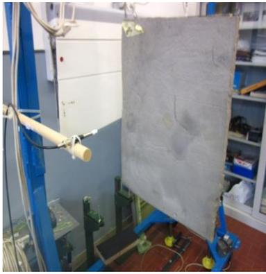
Fig. 15 Acoustic test set-up, Plate with Foam 65-30
