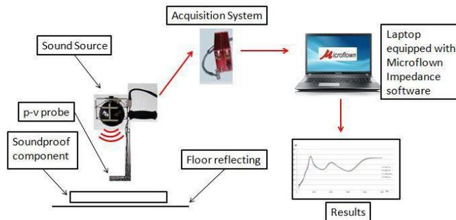
Fig. 33 PU probe, test setup
