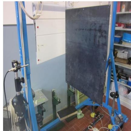
Fig. 13 Acoustic test set-up, Plate
