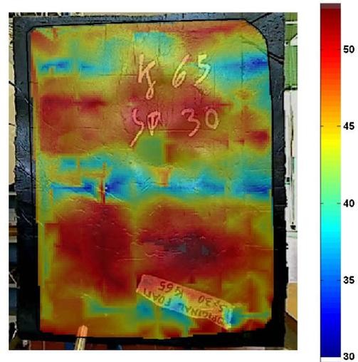
Fig. 35 Acoustic intensity, Original Foam
