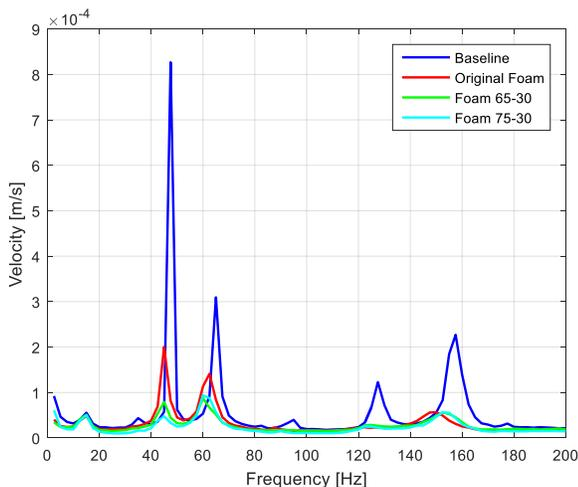
Fig. 3 Vibration velocity spectrum, Laser Test
