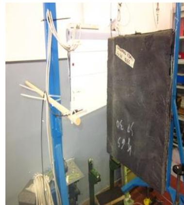
Fig. 14 Acoustic test set-up, Plate with Original Foam
