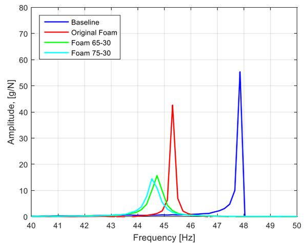
Fig. 8 Frequency Response Function (FRF), first mode detail
