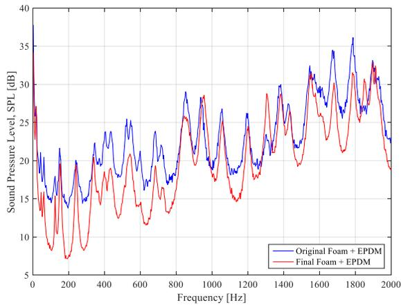
Fig. 42 Sound Pressure Level (SPL) spectral distribution
