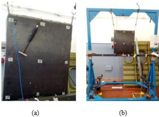
Fig. 6 Vibration test set-up: instrumentation (a), test rig (b)
