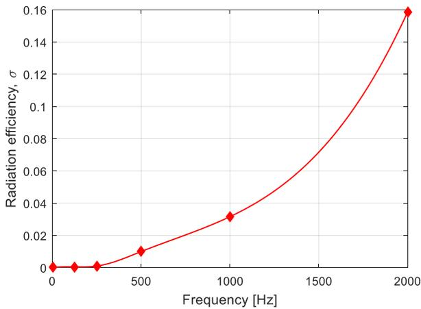
Fig. 19 Radiation efficiency: steel plate (0.5\*0.5\*0.0015 m)
