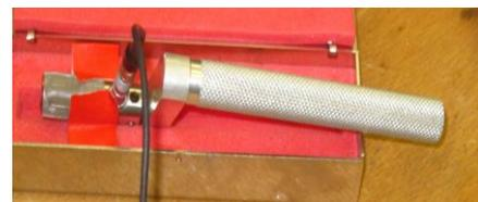
Fig. 31 PU probe, Microflown Technologies®
