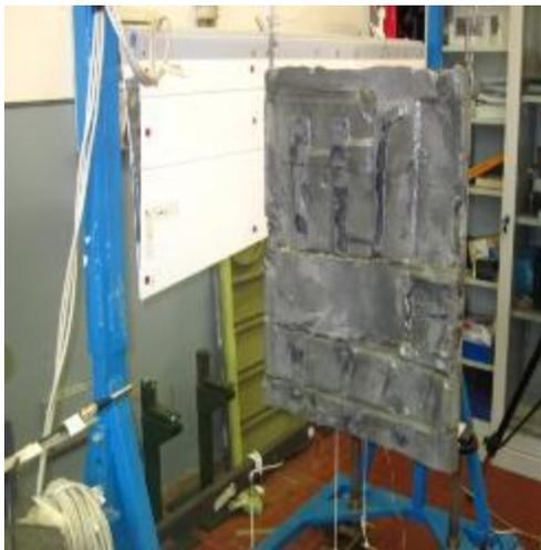
Fig. 24 Acoustic test set-up, Plate with foam prototype
