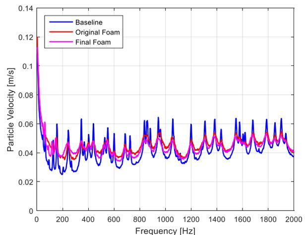
Fig. 32 Particle velocity by means of PU probe
