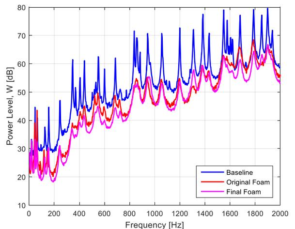
Fig. 27 Radiated sound power
