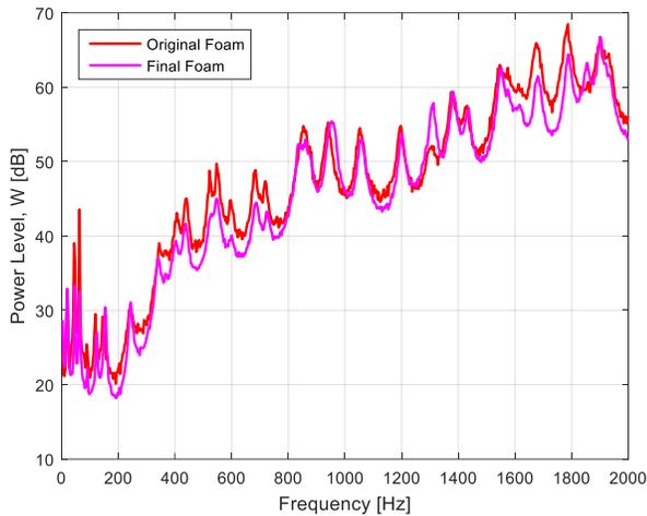
Fig. 28 Radiated sound power: foams behavior trade-off
