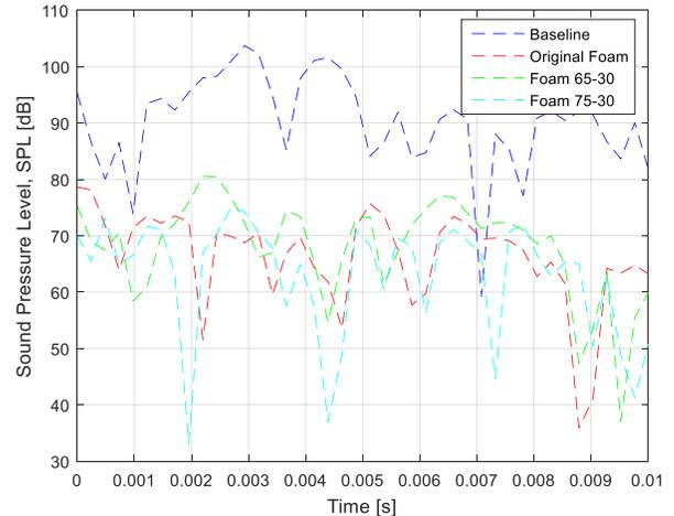
Fig. 18 Sound Pressure Level (SPL), time domain
