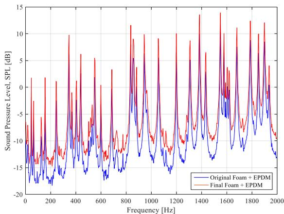
Fig. 43 Insertion Loss evaluation
