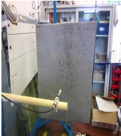
Fig. 16 Acoustic test set-up, Plate with Foam 75-30
