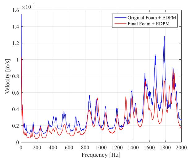
Fig. 40 Vibration velocity spectrum, Laser Test
