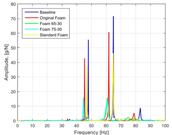
Fig. 22 Frequency Response Function (FRF) of different tested configurations
