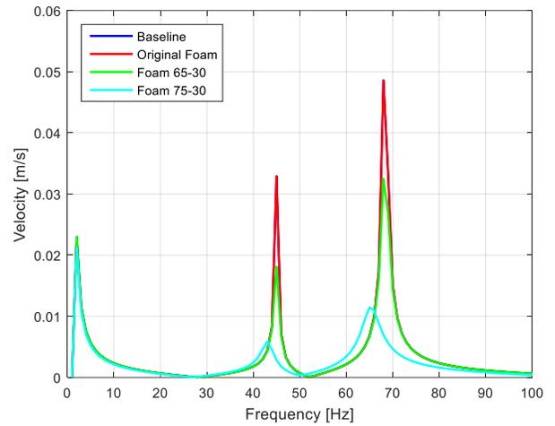
Fig. 12 Vibration velocity spectrum, SOL 111
