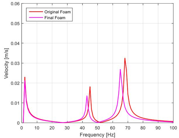
Fig. 30 Vibration velocity spectrum, SOL 111
