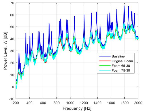
Fig. 21 Radiated sound power, range [200; 2000 Hz]
