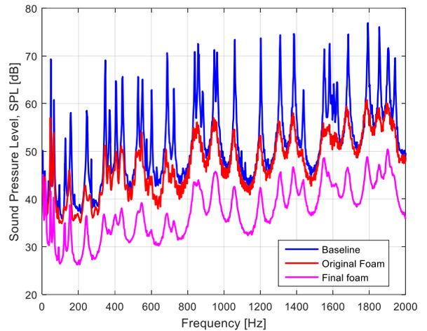
Fig. 25 Sound Pressure Level (SPL) spectral distribution
