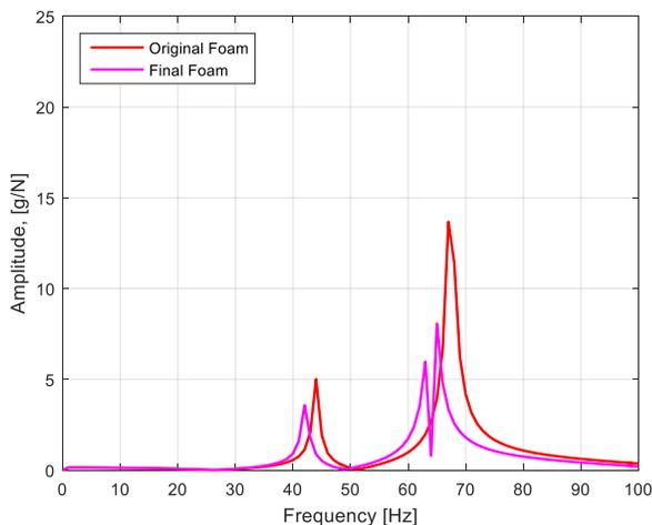
Fig. 29 Frequency Response Function (FRF), SOL 111
