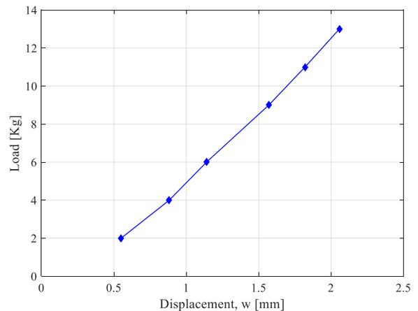
Fig. 36 Load-Displacement curve, Compression test
