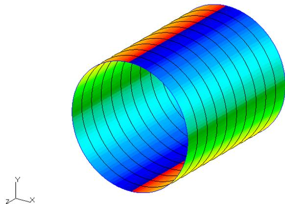
Fig. 8 External tonal load field
