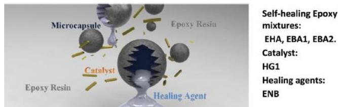
Fig. 2 Different compositions of self-healing systems [2]
