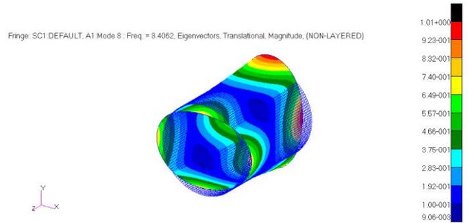
Fig. 12 Structural frame: third mode shape
