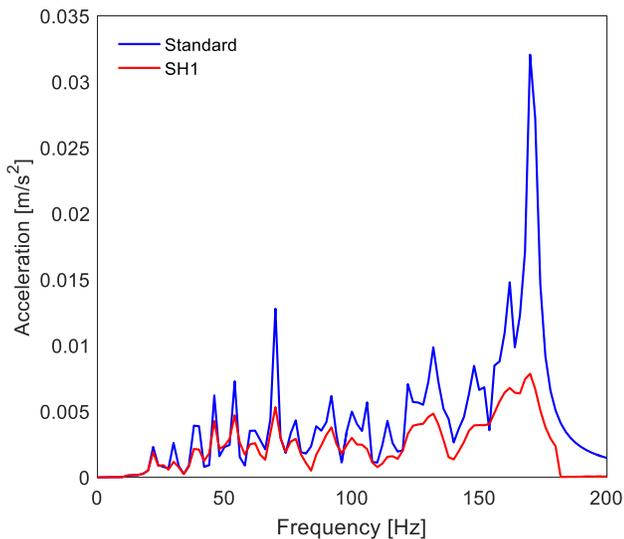
Fig. 15 Vibration acceleration spectrum, SOL 111
