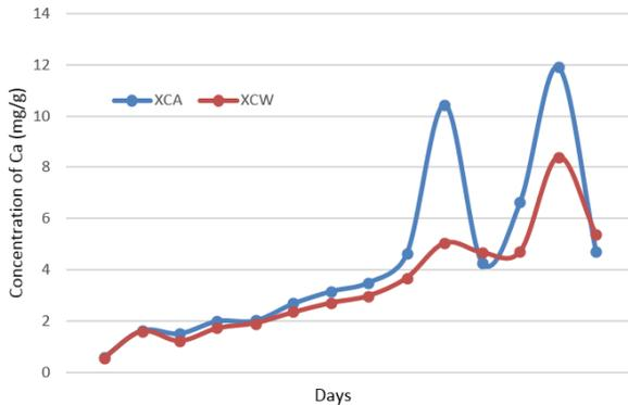
Fig. 2 Ca dissolving trend due to diluted bacterial environment II
