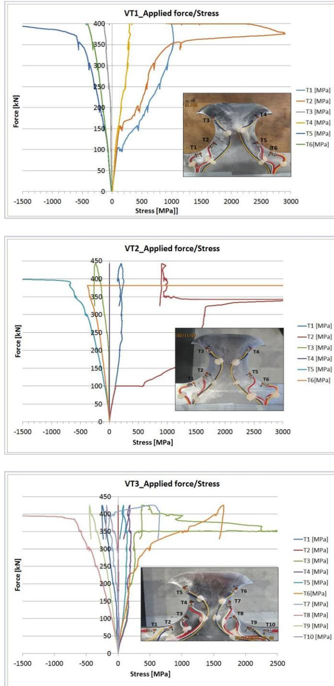
Fig. 13 the force/stress diagrams, test specimen VT1, VT2, VT3
