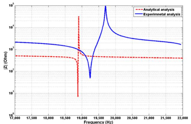
Figure 4. Impedance curve from analytical and experimental
