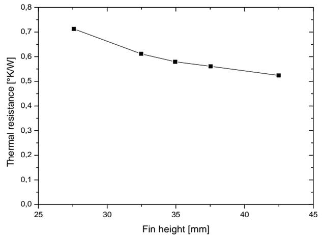
Fig. 6 The dependence of thermal resistance on the fin height for 65 fins, z/D = 8, Re = 15000, and fin width = 2.64 mm.
