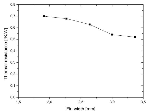
Fig. 7 The dependence of thermal resistance on the fin width for 65 fins, z/D = 8, Re = 15000, and fin height = 32.5 mm.
