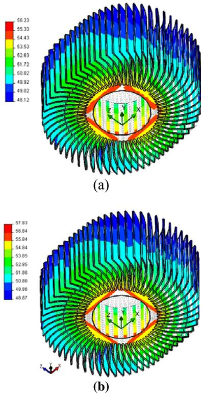
Fig .8 Grid independent solution: Temperature distributions through the heat sink, (3D).
