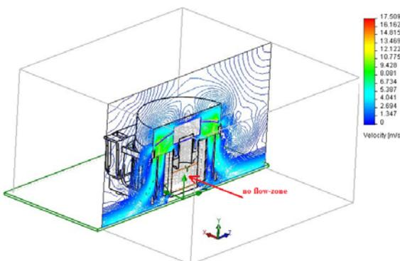
Fig. 10 Velocity vectors distribution
