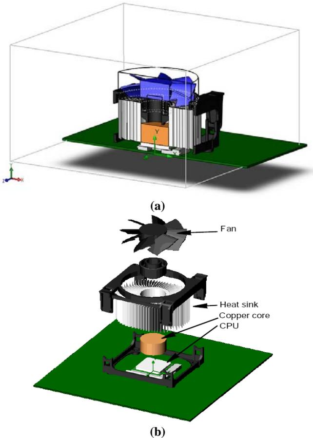
Fig.1 Schematic diagram showing the physical model: (a) Overall drawing, (b) exploded drawing.
