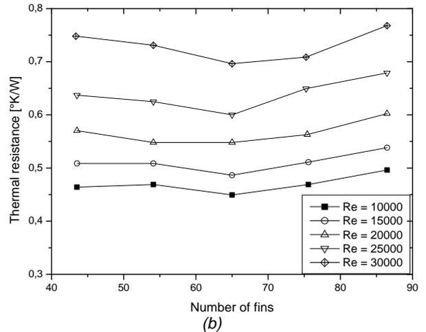
Fig. 5 (a) Thermal resistance of the heat sink based on various grids for Re = 15520, (b) Thermal resistance vs. number of fins at various Reynolds numbers.
