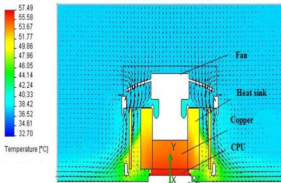
Fig .9 Temperature field and velocity vectors distribution
