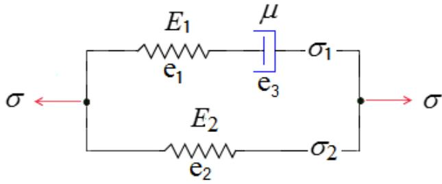
Fig. 4. Rheological model for standard linear model.
