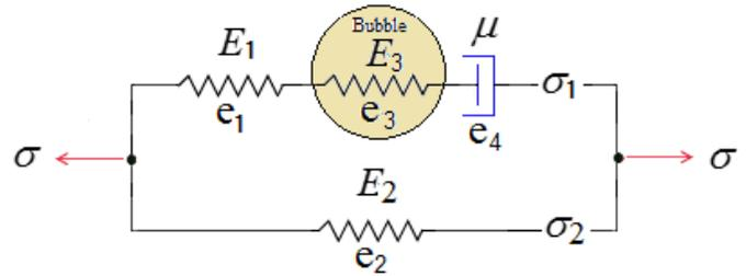
Fig. 3. A simplified rheological model including the bubble.
