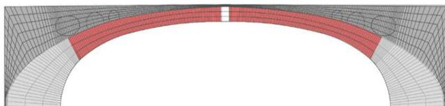
Figure 3: Model of the bridge with vault/tympanum/lightened fill assemblage.
