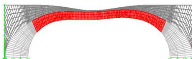
Figure 14: Deformed configuration of the 2D assembled system without holes under the coupled action of the self-weight and accidental loads.
