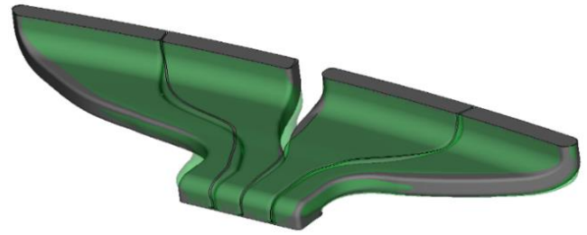
Fig. 7 Result of optimization of the air duct geometry (grey - initial geometry, green - optimized)
