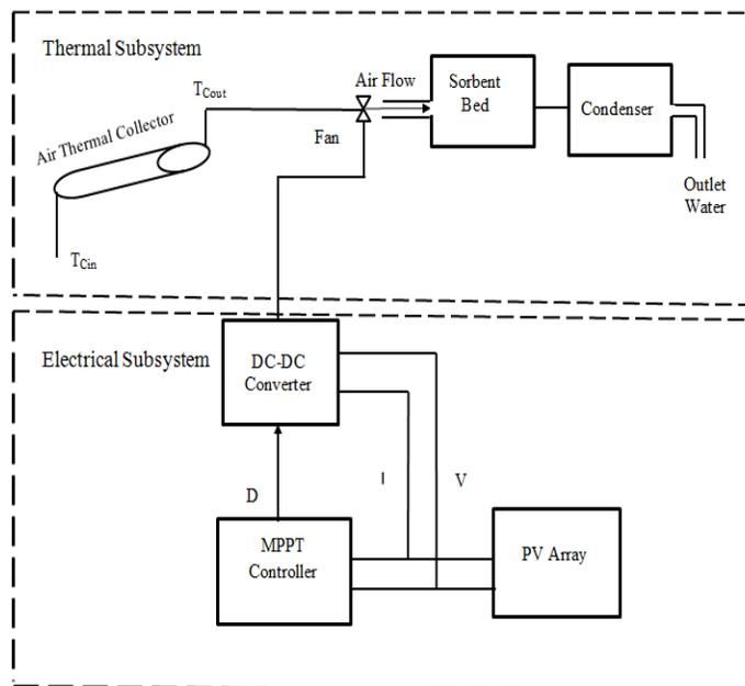
Fig.7 proposed water from air production system
