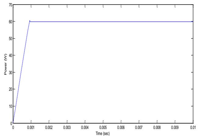
Fig. 24 P&O algorithm time response of PV array output power under 1000W/m<sup>2</sup> and 25°C
