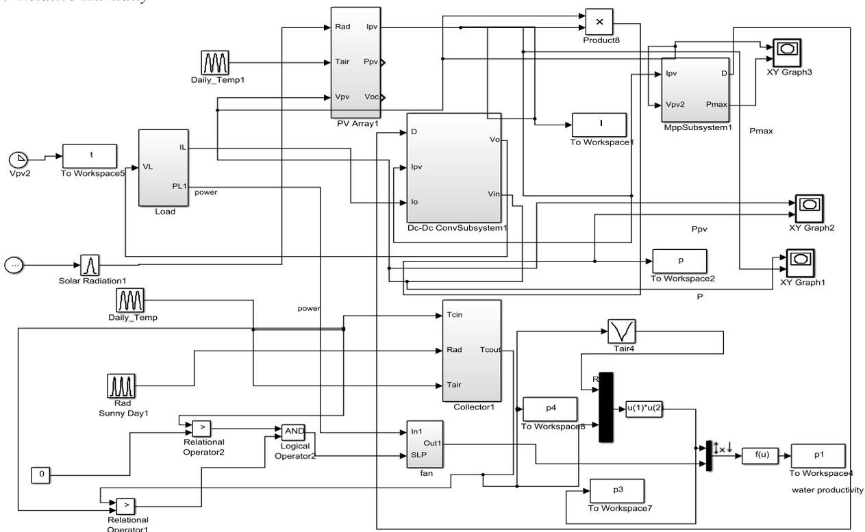
Fig.10 Simulink block diagram of water production system
