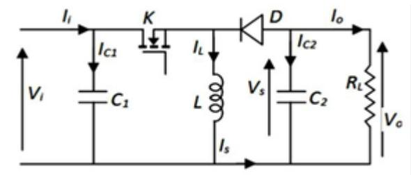
Fig. 8 Boost converter topology
