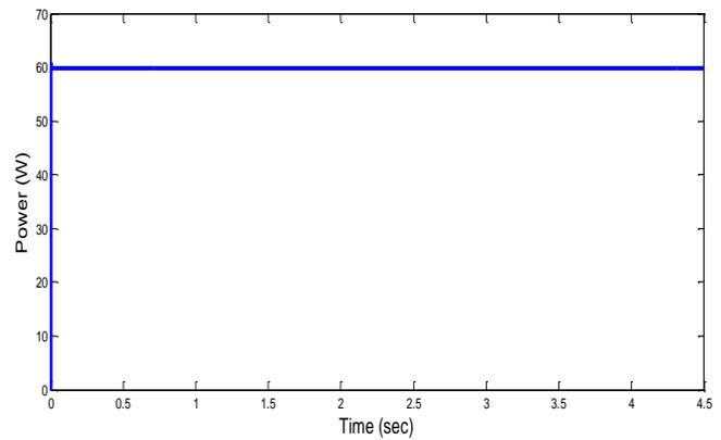
Fig. 23 PV array output power under 1000W/m<sup>2</sup> and 25°C
