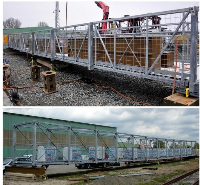
Fig. 5 full-scale testing of the “short” footbridge (on the top) and of the “long” footbridge (on the bottom)
