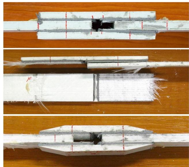
Fig. 15 failed specimens (an example of the specimen with skewed edges of the cover adherents is on the bottom)
