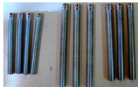
Fig. 6 some prepared specimens for the load tests
