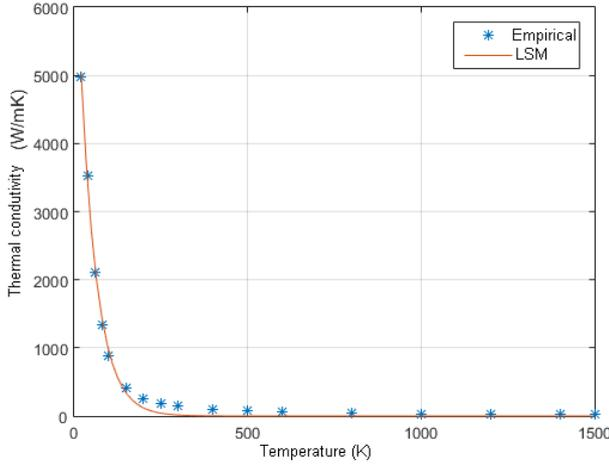
Fig. 2: Curve fitting by LSM in exponential type.
