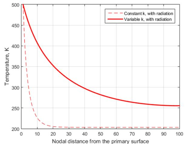
Fig. 4: Thermal profile of single fin, with radiation and variable  $k$
