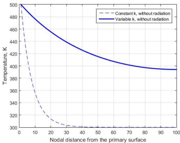
Fig. 3: Thermal profile without radiation and variable  $k$ .
