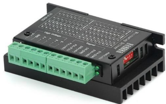
Fig. 5. TB6600 stepper motor driver
