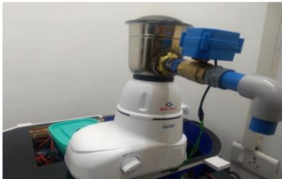
Fig. 1. Mixer-Grinder with Motorized Valve
