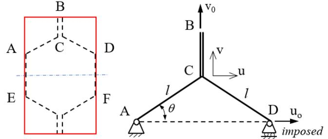
Fig. 3. Model for calculating elastic modulus  $E_x$  for a REV of honeycomb core
