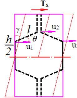
Fig. 4. Calculation model of shear modulus  $G_{xy}$  for a REV of honeycomb core
