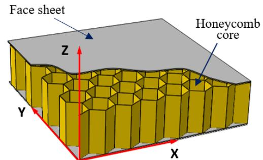
*Fig. 1 Honeycomb core sandwich plate model*
