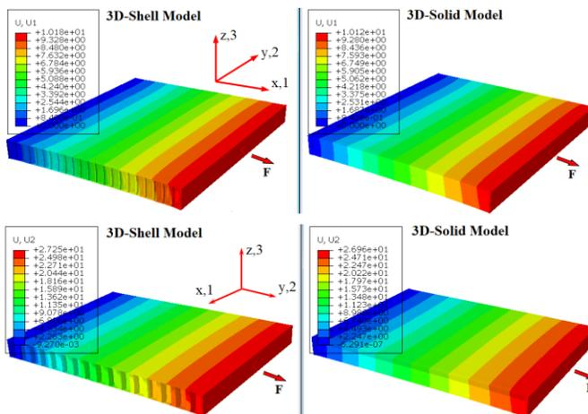
Fig.8. Simulation of 3D-Shell model and 3D-Solid model in traction for the honeycomb core sandwich
