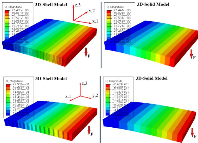
Fig.10. Simulation of 3D-Shell model and 3D-Solid model in bending and shearing coupling for the honeycomb core sandwich
