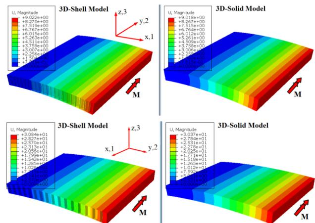
Fig.9. Simulation of 3D-Shell model and 3D-Solid model in pure bending for the honeycomb core sandwich
