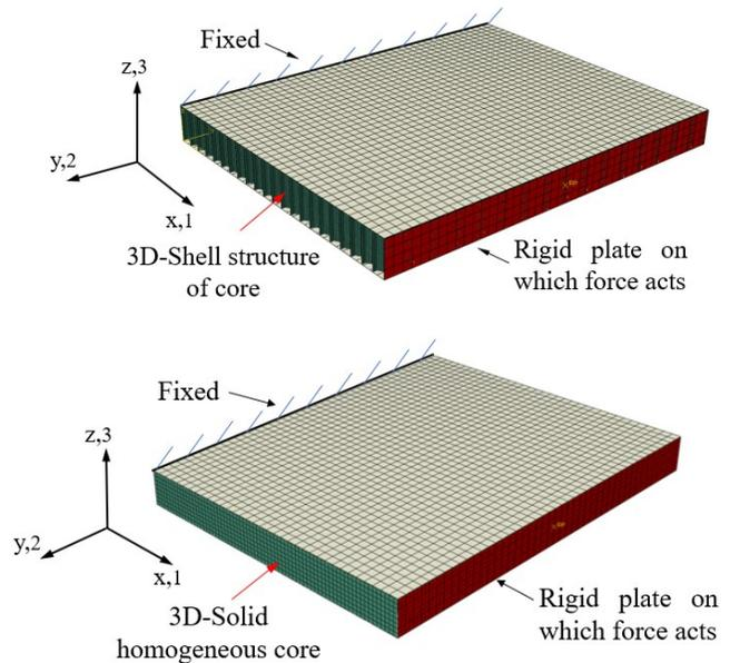
Fig. 7. Boundary conditions of 3D-shell plate and 3D-solid plate used for the simulations.
