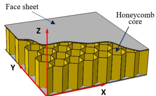
*Fig. 1 Honeycomb core sandwich plate model*
