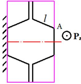
Fig. 5. Calculation model of shear modulus  $G_{xz}$  for a REV of honeycomb core
