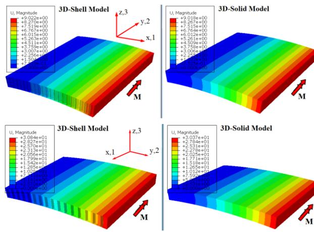
Fig.9. Simulation of 3D-Shell model and 3D-Solid model in pure bending for the honeycomb core sandwich
