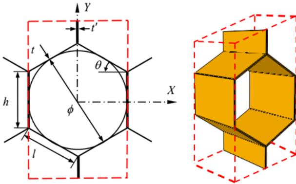
Fig. 2. Representative volume elemental (RVE) for honeycomb core
