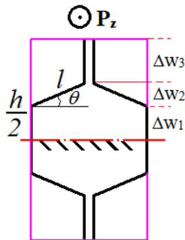
Fig. 6. Calculation model of shear modulus  $G_{yz}$  for a REV of honeycomb core
