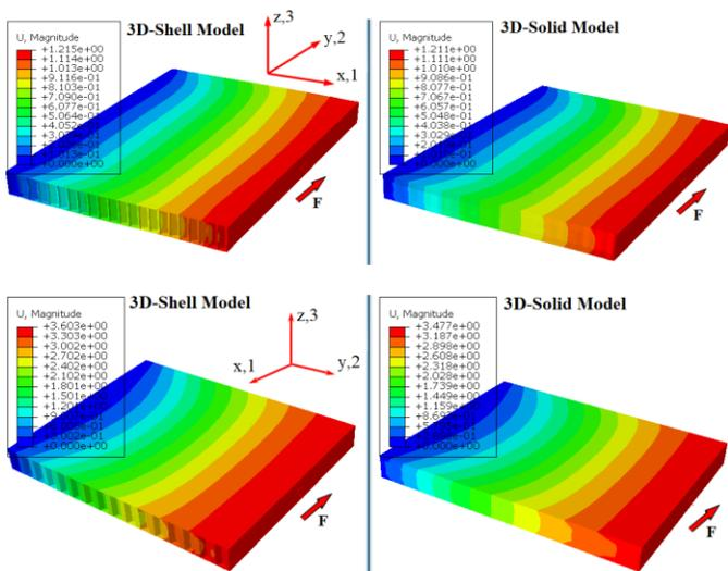
Fig.11. Simulation of 3D-Shell model and 3D-Solid model in in-plane shear for the honeycomb core sandwich
