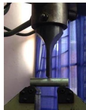
Fig. 3 Three bending point testing
