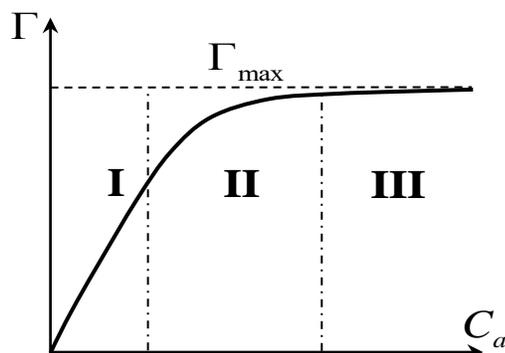
Fig. 1 Adsorption isotherm and its characteristic regions.
