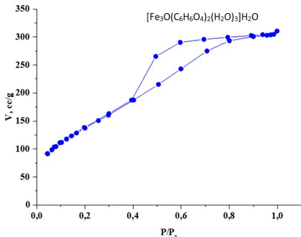
Fig. 5 Adsorption - desorption isotherms of nitrogen for the obtained coordination polymer.
