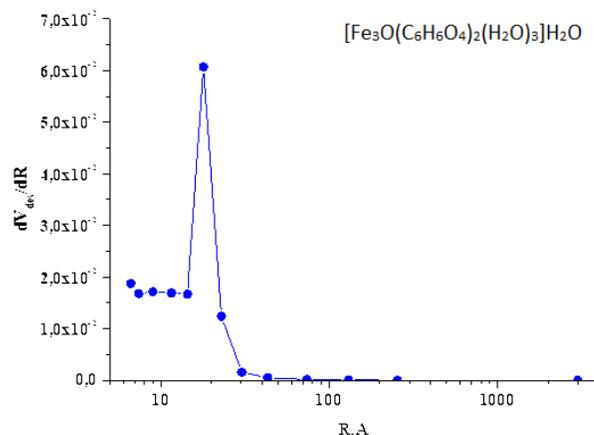
Fig. 6 Differential distribution curve of pore volume along the radii  $r$ .
