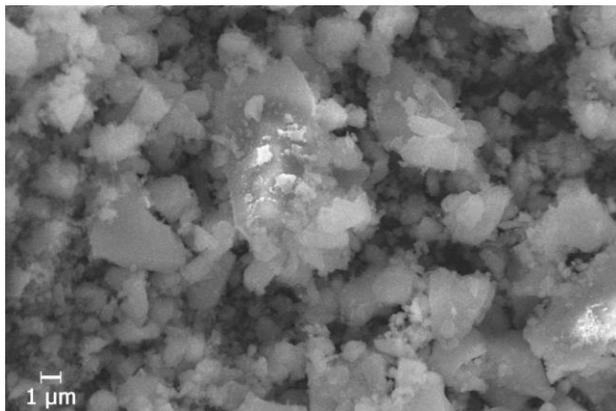
Fig. 4 sem micrographs of the coordination polymer.
