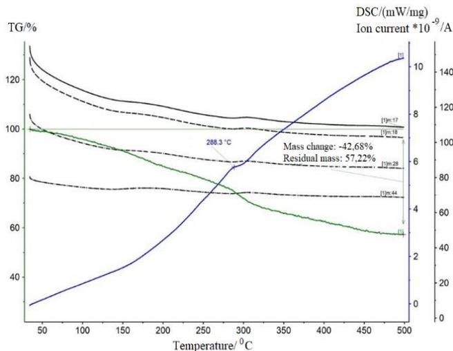
Fig. 2 Thermogravimetric analysis of the obtained coordination polymer combined with differential scanning calorimetry.
