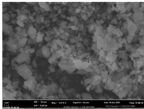
Fig. 3 sem photomicrographs of tricyclic iron acetate.
