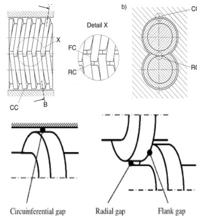
Fig. 7: Gap leakages; CC-Circumferential, RC-Radial, FC-Flank, (top) [19]; (bottom) [20]
