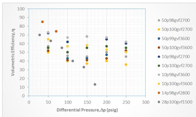
Fig. 6: Multiphase Twin Screw Pump performance in the neighborhood of 100% GVF
