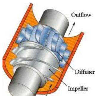
Fig. 2: Typical Helico-Axial Multiphase Pump [10]
