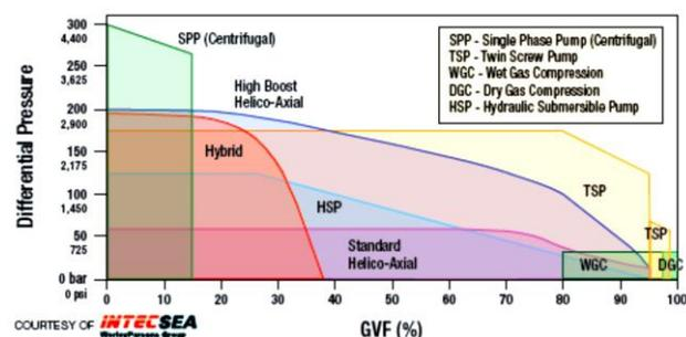
Fig. 1: Boundaries of sub-sea pumping applications (from [4])
