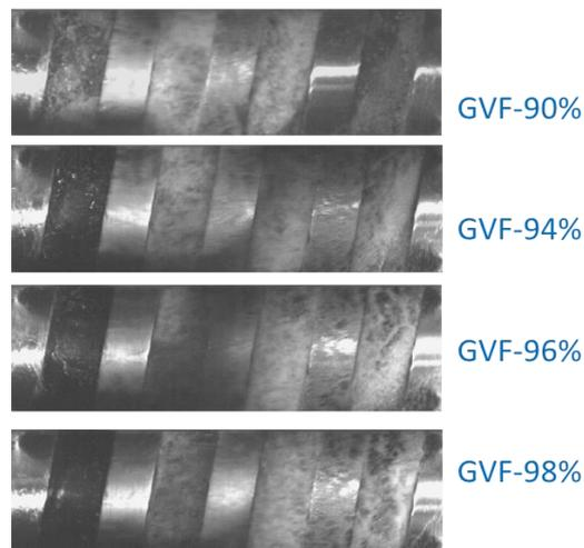
Fig. 9: Typical flow characteristics in perimeter gap [20]
