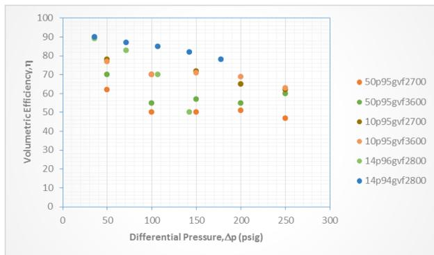
Fig. 5: Multiphase Twin Screw Pump performance in the neighborhood of 95% GVF
