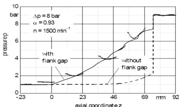
Fig. 8: Actual pressure rise with flank leakage and calculated pressure rise without flank leakage [29]
