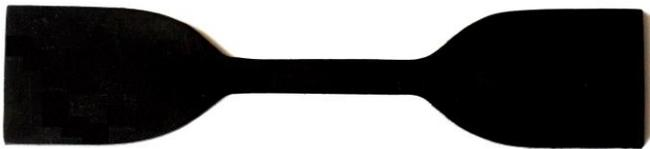
Fig. 5 1A type of uniaxial tension test specimen (according to ISO 37)
