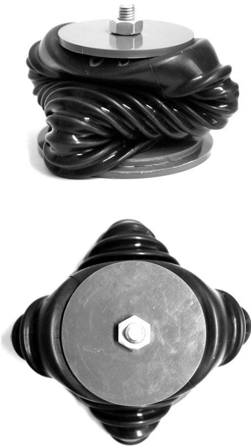
Fig. 3 buckling of the boot with an inappropriate profile ( $h=1.8$  mm)
