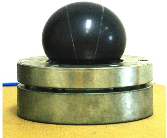
Fig. 9 equibiaxial tension test
