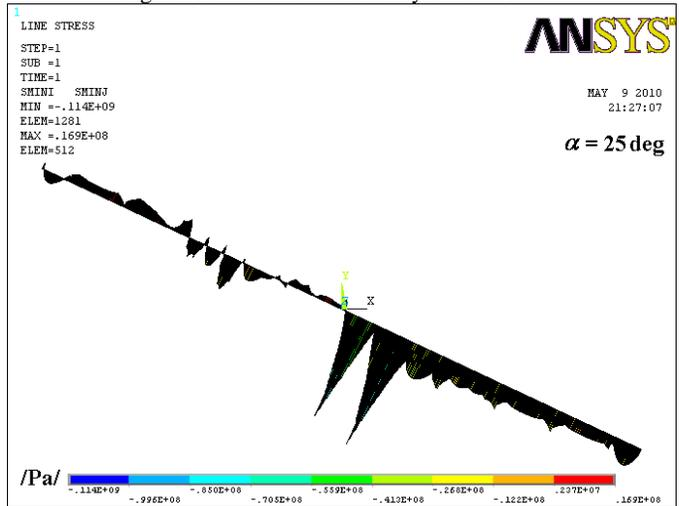
Fig. 20 Stresses in the rails and anchor pins of rack-railway track in mines (ANSYS sw)
