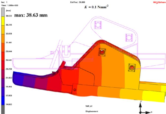
Fig. 17 Mechanical contact between mining supports and foot-wall approximated via elastic foundation (total displacement, MSC.MARC/MENTAT sw)
