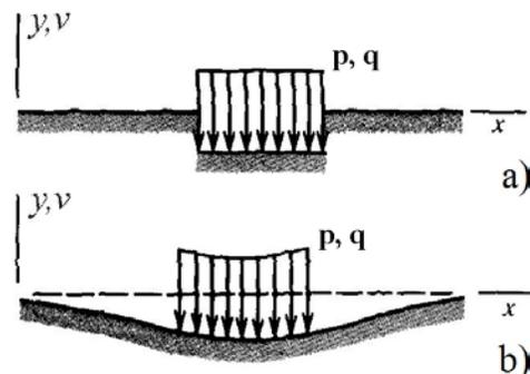
Fig. 2 Deflection of structure on elastic foundation under pressure  $p$  or distributed loading  $q$ , (a) Winkler foundation, (b) elastic solid foundation
