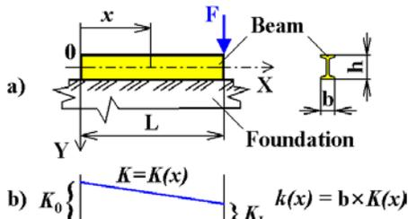
Fig. 8 Solved beam on elastic variable foundation
