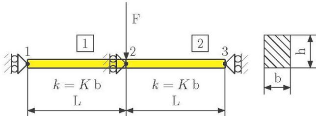
Fig. 4 FE model using BEAM54, see [10]
