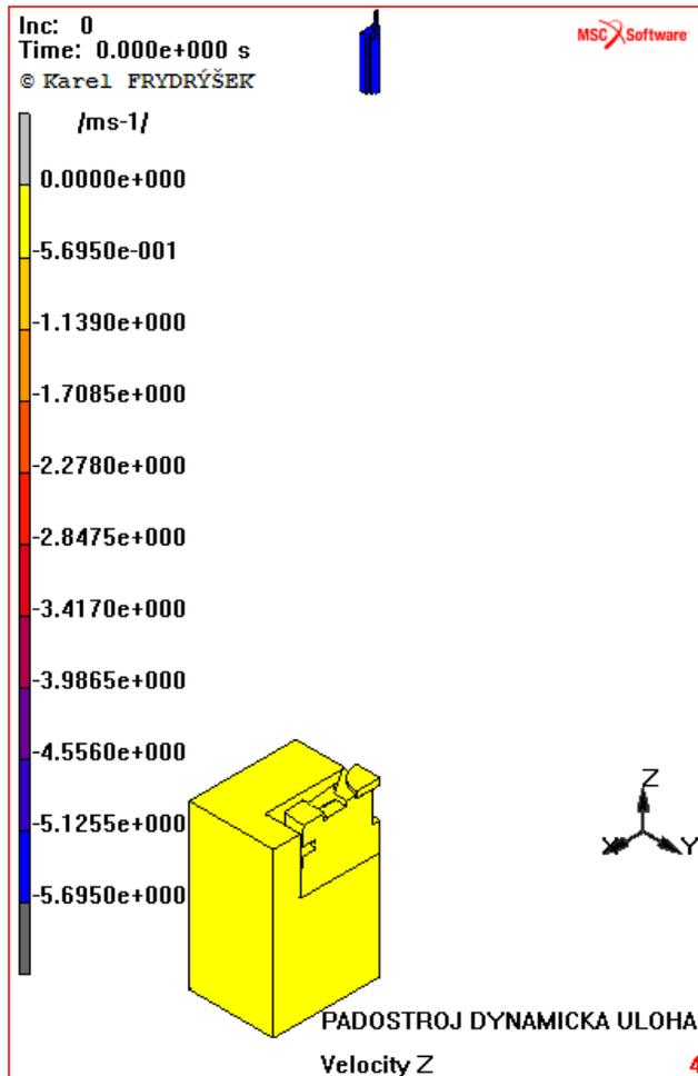
Fig. 21 Calculations of dynamic forces in the foundations of a massive drop-tester during impact tests (3D body on elastic foundation, MSC.MARC/MENTAT sw)
