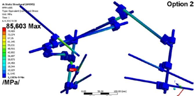
Fig. 15 “Option 2” – Finite Element modelling of the external fixator for treatment of pelvis and its acetabulum (equivalent von Mises stresses /MPa/ for tensile loading 100 N)
