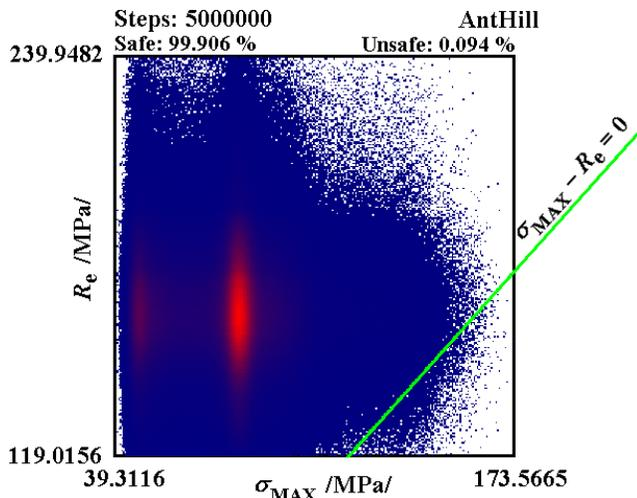
Fig. 12 2D histogram of output parameters (calculation of  $F_s$  - probabilistic reliability assessment)
