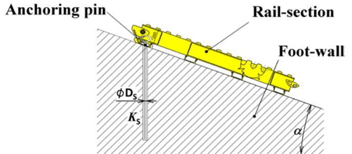
Fig. 19 Problem - Rack-railway track in mines
