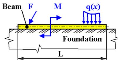
Fig. 1 Example of a beam resting on an elastic foundation. This beam is loaded by force  $F$ , couple  $M$  and distributed loading  $q$ .
