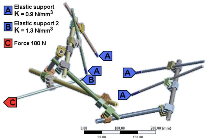
Fig. 14 External fixator for treatment of pelvis and its acetabulum - FE model, boundary conditions (A, B is applied elastic foundation, Ansys sw)
