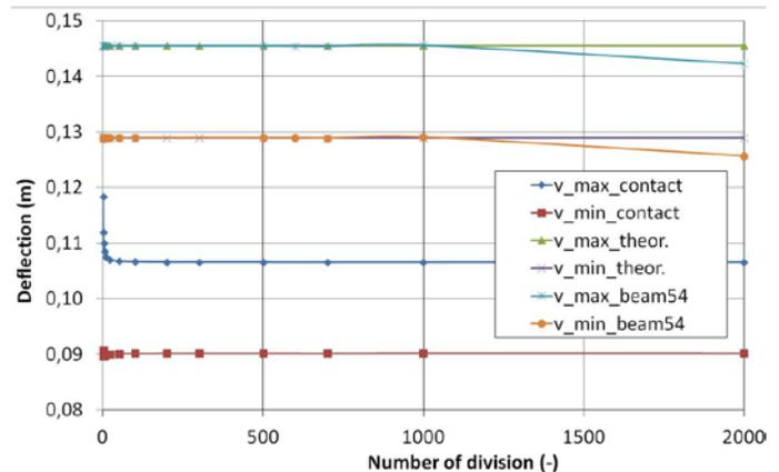
Fig. 6 The influence of number of element divisions along the length  $L$  on the minimum and maximum deflection, see [10]
