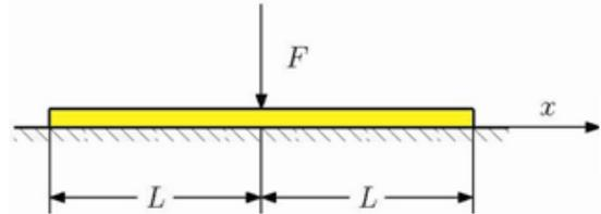
Fig. 5 Beam on elastic foundation (solved example)
