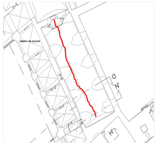
Fig. 5 - The Chapter Hall plan with the main crack in the key; one may notice the resistant panels facing the main cloister with a free length of about 40 m.
