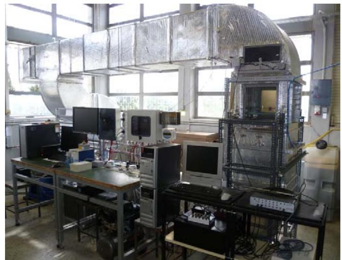
Fig. 2 Photo of the LC dryer, equipped with measuring instrumentation and data acquisition system
