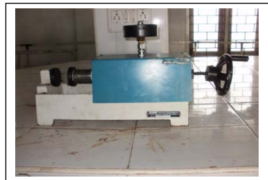
(b) Universal sand testing machine
